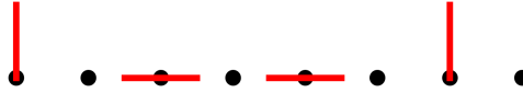
Fig. 1.: Lattice-gas representation of “dimers”. The lattice-gas model considers all particles to occupy a single lattice site. Dimers which lie parallel to the surface should occupy two lattice sites.
