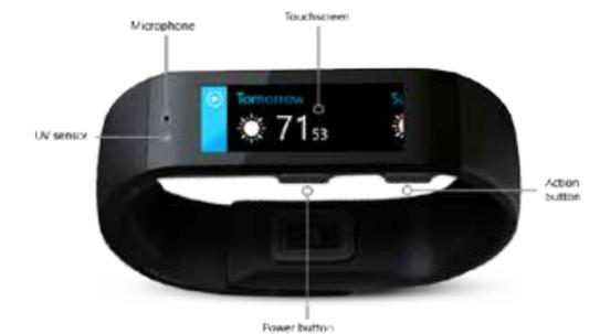
The Microsoft Band biometric technology worn by the lab's test subjects measures step counts, sleep quality, heart rate and other physical data while the lab's scientists remotely control various "scenes" in typical office and living environments (Source: microsoft.com).
