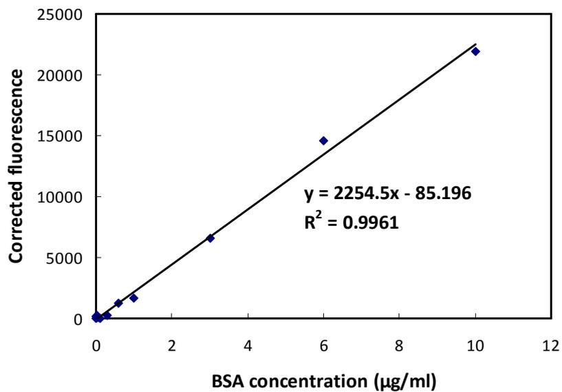
Figure 2.10. The standard curve of the NanoOrange® protein assay.
