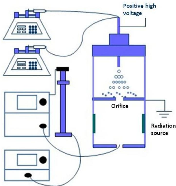
Figure 2.3. A schematic diagram of the electro spray close system along with a Scanning Mobility Particle Sizer (SMPS) to characterize size distributions of ES PLGA nanoparticles.
