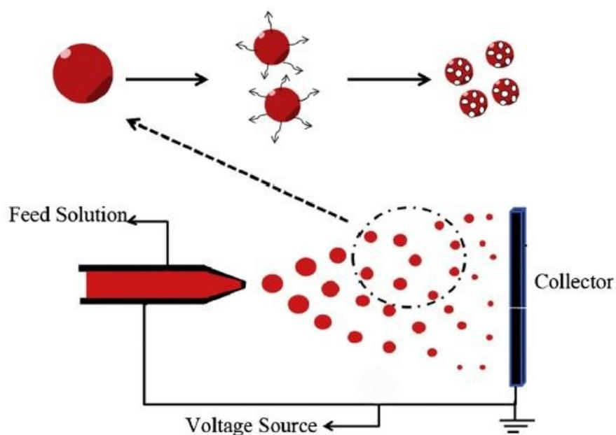
Figure 2.1. A schematic representation of a typical electro spray setup with the point-to-plate configuration [Hao et al., 2014].
