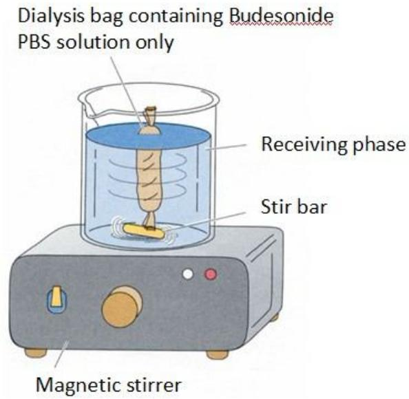
Figure 2.4. A schematic diagram of the dialysis apparatus for studying diffusion of Budesonide across the dialysis membrane.
