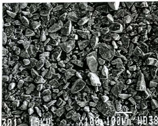
Figure AVI.1 SEMs of (a) “coarse fraction” and (b) “fine fraction” of lactose.
