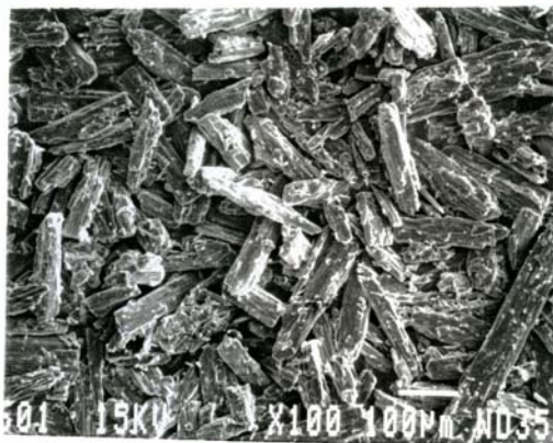
Figure AVI.4 SEMs of (a) “coarse fraction” and (b) “fine fraction” of mannitol.
