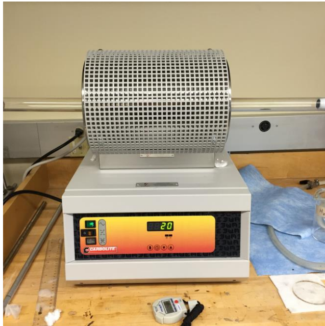
Figure 3-2: Photography of the tubular furnace
