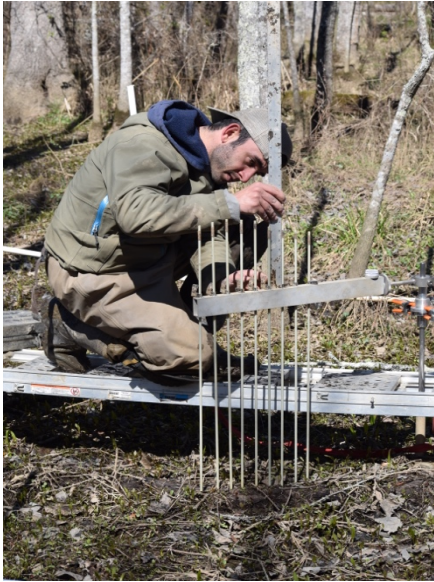
Figure 4 Measuring the SET instrument in James River NWR. The pins have been locked into place at sediment surface, and we are measuring from the top of the pins to the top of the arm.
