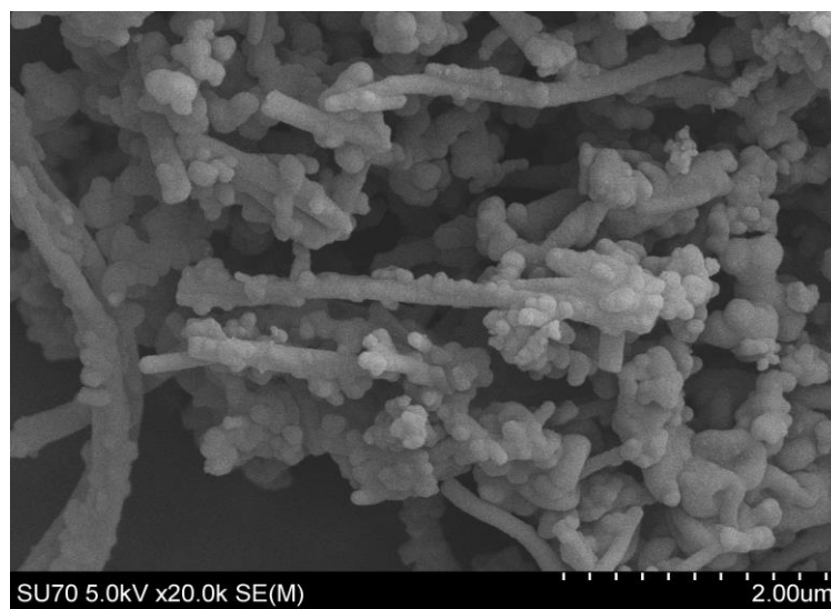
Figure 4.4: Scanning electron microscopy (SEM) image of Azo-Py
