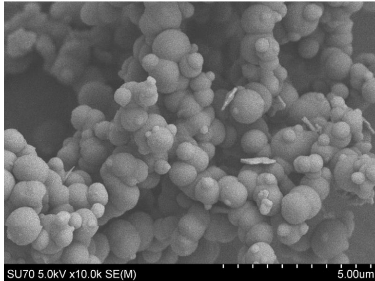
Figure 3.4 (a): Scanning electron microscopy (SEM) images of BILP-30
