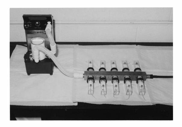
aerosolized mist from the nebulizer chamber to an exposure chamber where the noses and mouths of the restrained test animals were exposed to the mist (exposure chamber and mouse restrainers designed and constructed by Misters E. Talley and E. M. Dimen, Dept. of Pharmacology). The mist was vented through a carrier hose attached to an aspirator and discharged into a sink.
