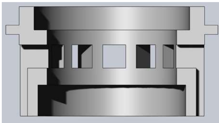
Figure 3.7: Section view of the second version of the strainer insert.
