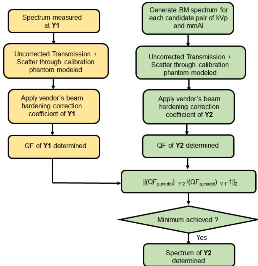
Fig.4.7. Flowchart of the proposed method of spectrum derivation based on BH polynomials correction
