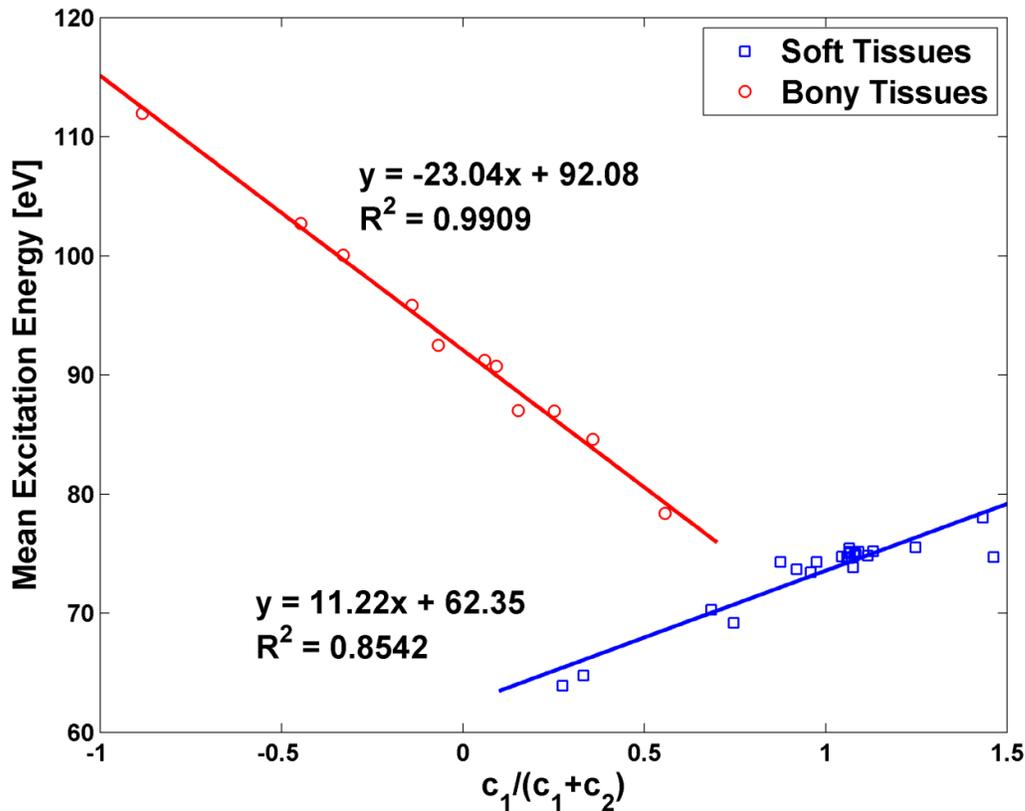
Fig. 2.2. The relationship between  $c_1/(c_1+c_2)$  and the I-values of 34 standard human tissues is shown. There are two separate linear fits, one for soft tissues and one for bony tissues. This relationship provides an alternative method to estimate I-value without knowing the  $Z^*$  of the substances. It was found the goodness of fit ( $R^2$ ) had minor impact on the achieved accuracy of proton stopping power estimation.
