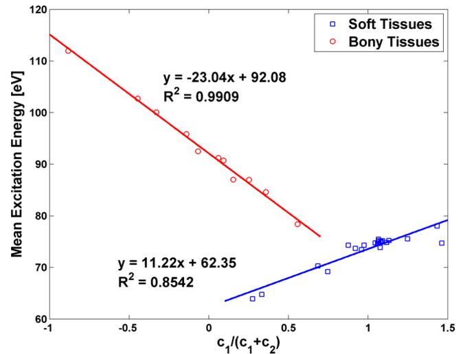
FIG. 10. The relationship between  $c_1/(c_1+c_2)$  and the  $I$ -values of 34 standard human tissue is shown. There are two separate linear fits, one for soft tissues and one for bony tissues. This relationship provides an alternative method to estimate  $I$ -value without knowing the  $Z^*$  of the substances.
