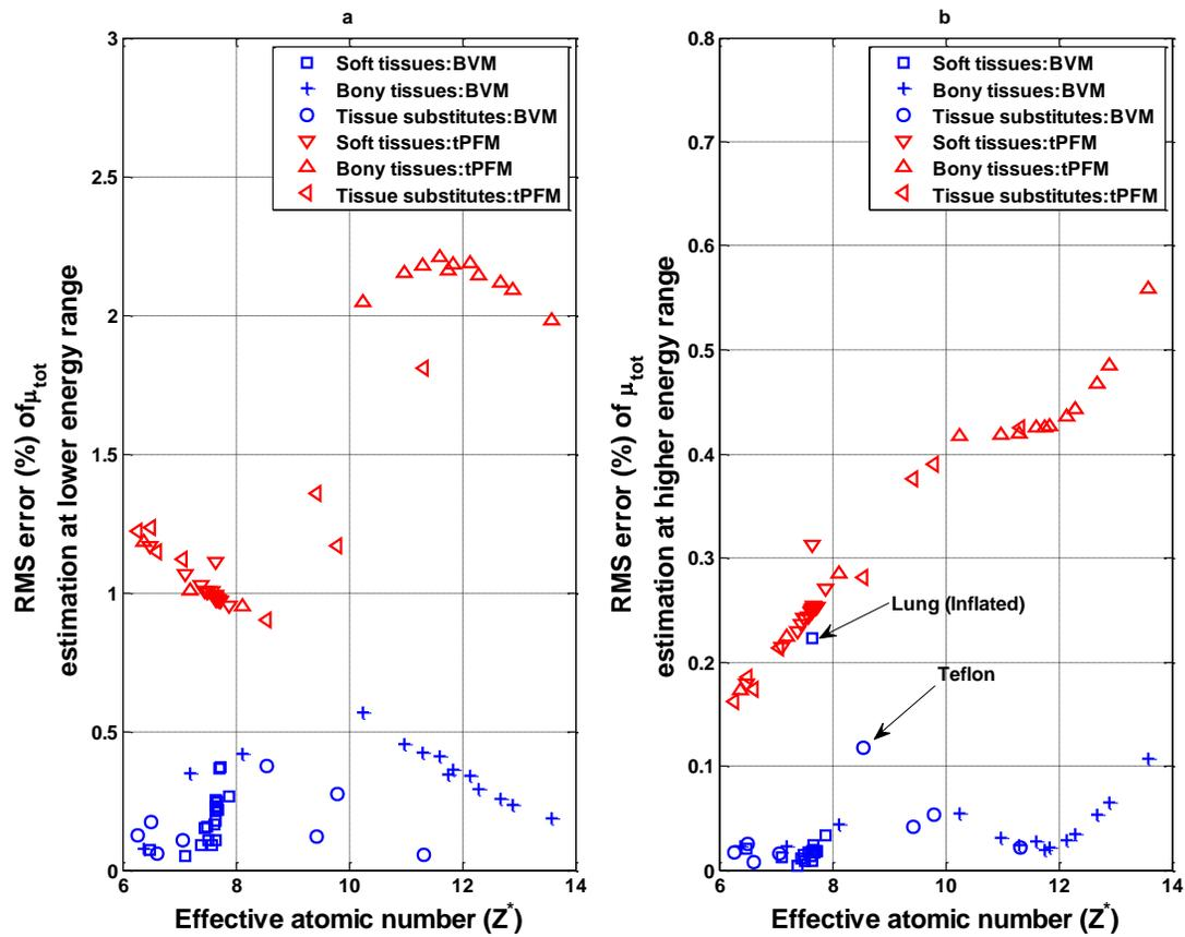
Fig. 3.1. Percent RMS error of the total linear attenuation coefficient predicted by BVM or tPFM for 43 tissues and phantom substitutes as functions of tPFM effective atomic number for the (a)  $20 \leq E \leq 50$  keV and (b)  $50 \leq E \leq 1000$  keV energy ranges. The thyroid tissue prediction error is outside the plotting range of the low energy plot.
