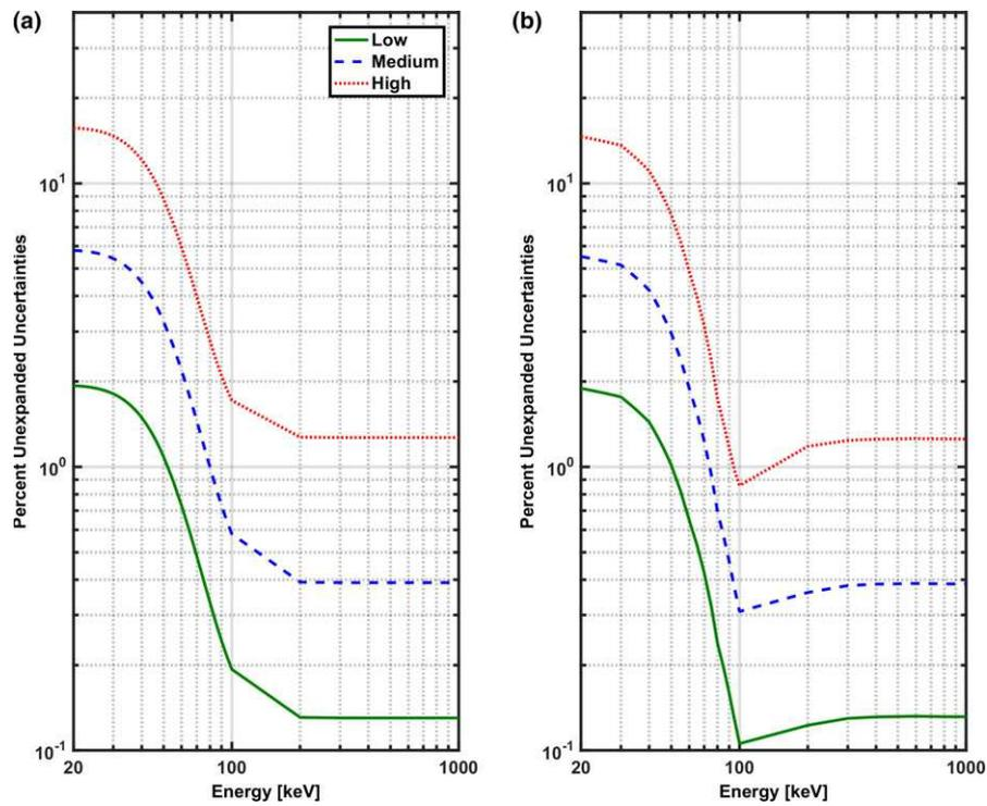
FIG. 6. Percent unexpanded uncertainty (coverage factor  $k = 1$ ) of the linear energy-absorption coefficient for PMMA as a function of energy for the (a) tPFM and (b) BVM models. The low, medium, and high curves denoted the uncertainties corresponding to the (low, high) energy image-intensity uncertainties (0.2%, 0.1%), (0.6%, 0.3%), and (1.5%, 1.0%), respectively. [Color figure can be viewed at [wileyonlinelibrary.com](http://wileyonlinelibrary.com)]
