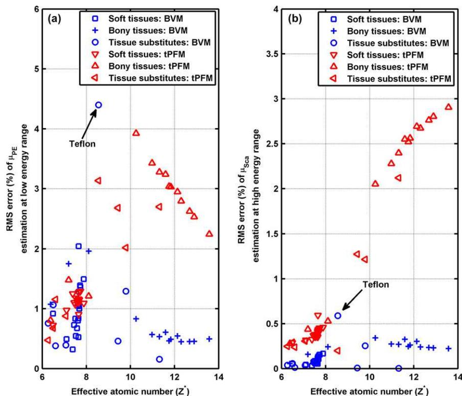
FIG. 2. tPFM and BVM percent RMS predictions for 43 tissues and phantom substitutes as functions of tPFM effective atomic number for (a) photoelectric effect cross-sections in the  $20 \leq E \leq 50$  keV range and (b) photon scattering cross-sections in the  $50 \leq E \leq 1000$  keV range. The thyroid tissue prediction error is outside the plotting range of the low-energy plot. [Color figure can be viewed at [wileyonlinelibrary.com](http://wileyonlinelibrary.com)]
