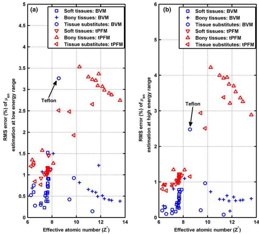
FIG. 3. Percent RMS error of energy-absorption coefficients estimate for 43 tissues and phantom materials as functions of tPFM effective atomic number for the (a)  $20 \leq E \leq 50$  keV and (b)  $50 \leq E \leq 1000$  keV energy ranges. The thyroid tissue prediction error is outside the plotting range of the low-energy plot. [Color figure can be viewed at wileyonlinelibrary.com]
