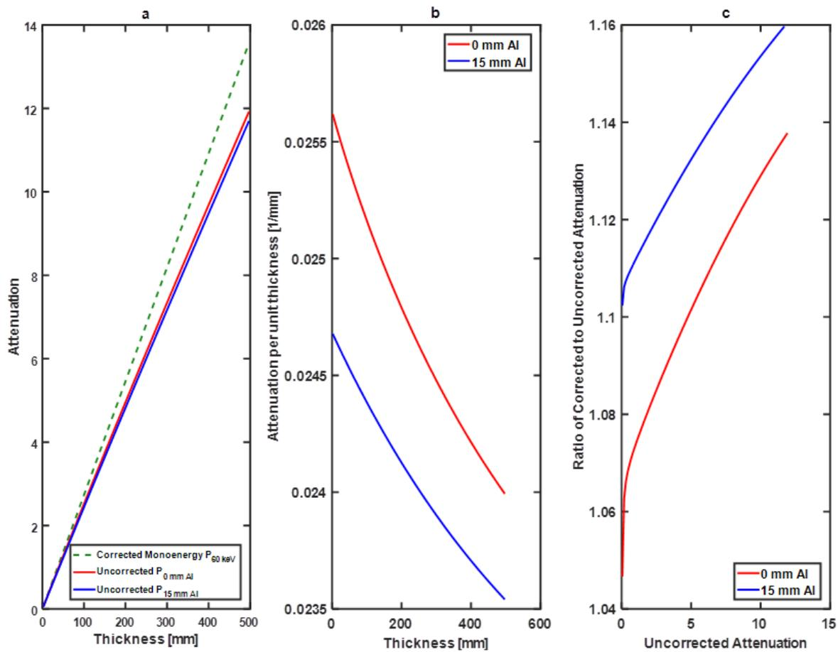
Fig. 4.3 illustration of BH water-based attenuation corrections for two different spectra passing through POM with varying thickness from 0 cm to 50 cm. (a) Uncorrected projections from spectra 0 mm Al and 15 mm Al and target monoenergetic (60 keV) projections; (b) Attenuation per thickness of two spectra, showing non-constant attenuation coefficient, i.e., beam-hardening effect; (c) ratios of corrected to uncorrected projections, showing the spectra dependent polynomial correction
