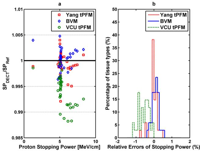
FIG. 5. (a) A comparison of errors in the stopping power predictions from different DECT models with reference values. The maximum relative error of prediction using the BVM was well below 0.5%. (b) The distribution of relative errors of the stopping power of 34 standard human tissues estimated by the BVM, Yang tPFM, and VCU tPFM is shown.
