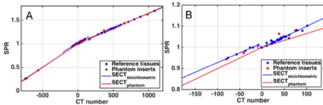
Fig.2.1 (A) Example of SECT stoichiometric calibration at 150 kVp using two linear segments implemented by Hudobivnik et al.<sup>108</sup>. Blue dots denote the tissues from ICRU reports, while red dots are for tissue phantom materials. (B) Enlargement of the soft tissue region. The stoichiometric calibration curves are obtained by plotting the HU and stopping power of phantom materials and tissues based on the procedure outlined in 2.1.1
