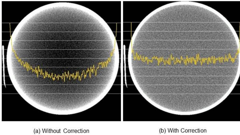
Fig. 4.2 (a) Cupping effects shown in the center region of 35-cm water phantom without correction applied (b) with BH correction scheme implemented, the BH artifacts nearly disappear.<sup>25</sup>
