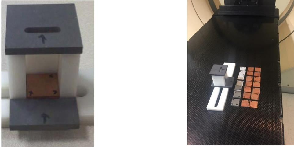
Fig.4.10. A collimator assembly<sup>98</sup> and stacks of Al and Cu are shown
