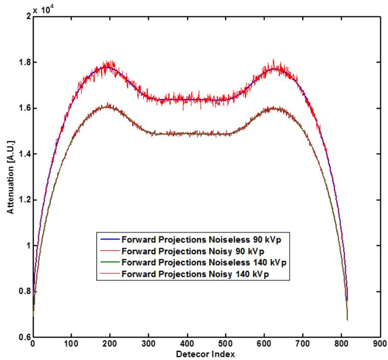
Fig.4.17 Comparisons of forward projections with and without noise for full calibration phantom at spectra of 90 kVp and 140 kVp.
