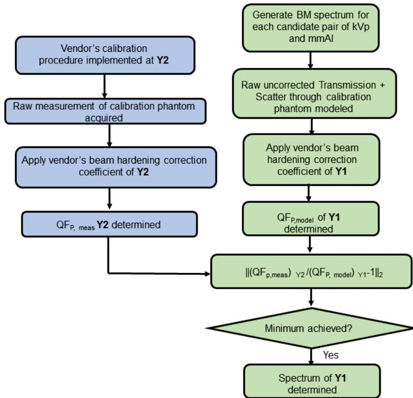
Fig.4.20. Flowchart of the method of spectrum derivation when a reference spectrum is not available
