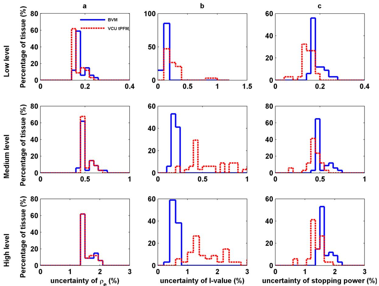
FIG. 8. The distribution of the uncertainties of 34 standard human tissues in electron density (a),  $I$ -values (b), and stopping power (c) from three different CT image uncertainty levels (low-, medium-, and high-level): top row: low level 0.2% and 0.1%; middle row: medium level 0.6% and 0.3%; and bottom row: high level 1.5% and 1.0%.
