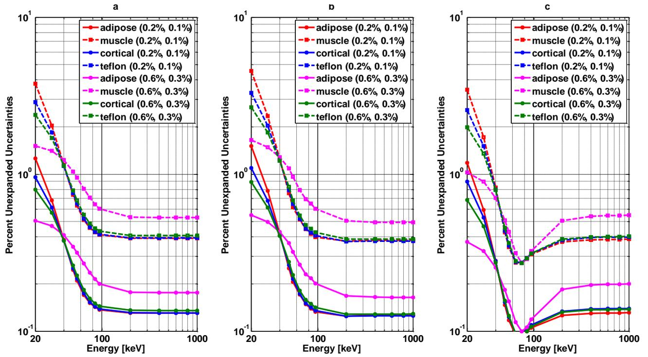
Figure S-F1. Percent unexpanded uncertainty of total linear attenuation for (a) tPFM, (b) vPFM and (c) BVM, respectively as functions of energy in the range  $20 \leq E \leq 1000$  keV, at image intensity uncertainty levels of (0.6%, 0.3%) and (0.2%, 0.1%) for (low, high) energy CT images. Four typical human tissues and tissue substitute were selected for analysis.
