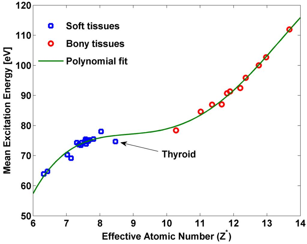
Fig.2.3 The polynomial relationship<sup>55</sup> between  $Z^*$  and mean excitation energy was implemented in the VCU tPFM. The fit of  $R^2$  is 0.9603. Data for 34 soft tissues and bony tissues are shown.
