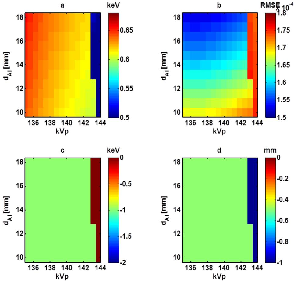
Fig.4.16 Comparisons of derived spectrum and independently simulated reference spectra for nominal 140 kVp with inherent filtration of aluminum ranging from 10 mm to 18 mm for the noiseless  $QF_{P,model}$ . The differences of mean energy (a), RMSE (b), kVp(c), and  $d_{Al}$  (d) are shown, respectively. Each pixel on the figures corresponded to the discrepancy for each candidate of spectrum.
