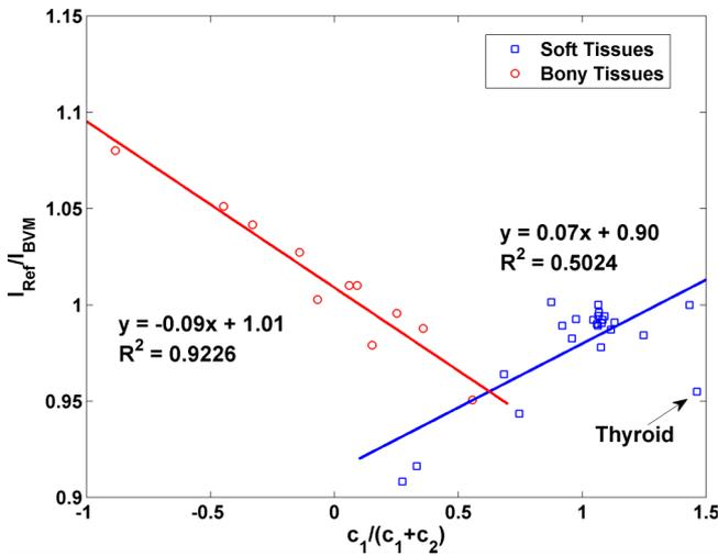
FIG. 2. The linear relationships between  $c_1/(c_1+c_2)$  and  $I$ -value prediction error by the BVM for soft tissues and bony tissues. This empirical function was used to correct the error of the  $I$ -value estimated by the BVM.
