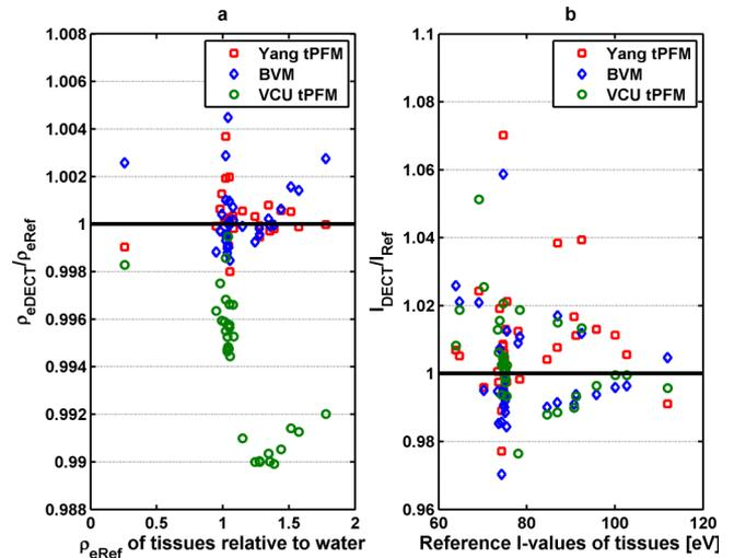
FIG. 4. The ratio of electron density and  $I$ -values estimation by three different models: the Yang tPFM, BVM, and VCU tPFM, respectively, to the reference value of stopping power. (a) Electron density and (b)  $I$ -values. The reference electron density of tissues is shown in the form of electron density relative to water. The reference  $I$ -values were computed based on the Bragg additivity rule.
