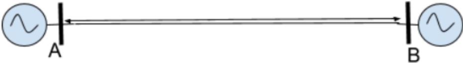
Figure 26: Two-terminal Transmission Line Details
