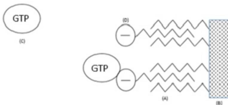
**Figure 3-6: Diagram of Ion Pairing RP-HPLC.** Ion pairing agents with hydrophobic tails (A) bind to the hydrophobic stationary phase (B). Polar molecules such as GTP or other nucleotides (C) bind to the polar end of the ion pairing molecules (D). Nucleotides elute from the stationary phase upon interaction with organic solvents due to disruption of the polar molecules. Detection of the nucleotides is accomplished by a UV sensor at 254 nm.
