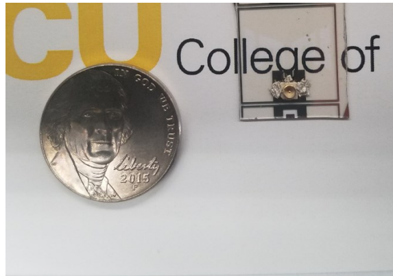
Figure 46 Fabricated 5.8 GHz Bowtie Slot Antenna.
