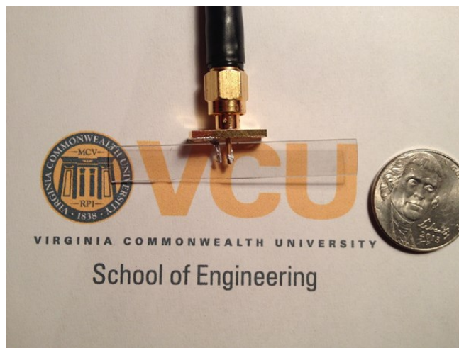
Figure 28 Fabricated 2.4 GHz transparent GZO Dipole Antenna.
