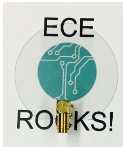
Figure 37 Fabricated 2.4 GHz GZO planar hourglass antenna.
