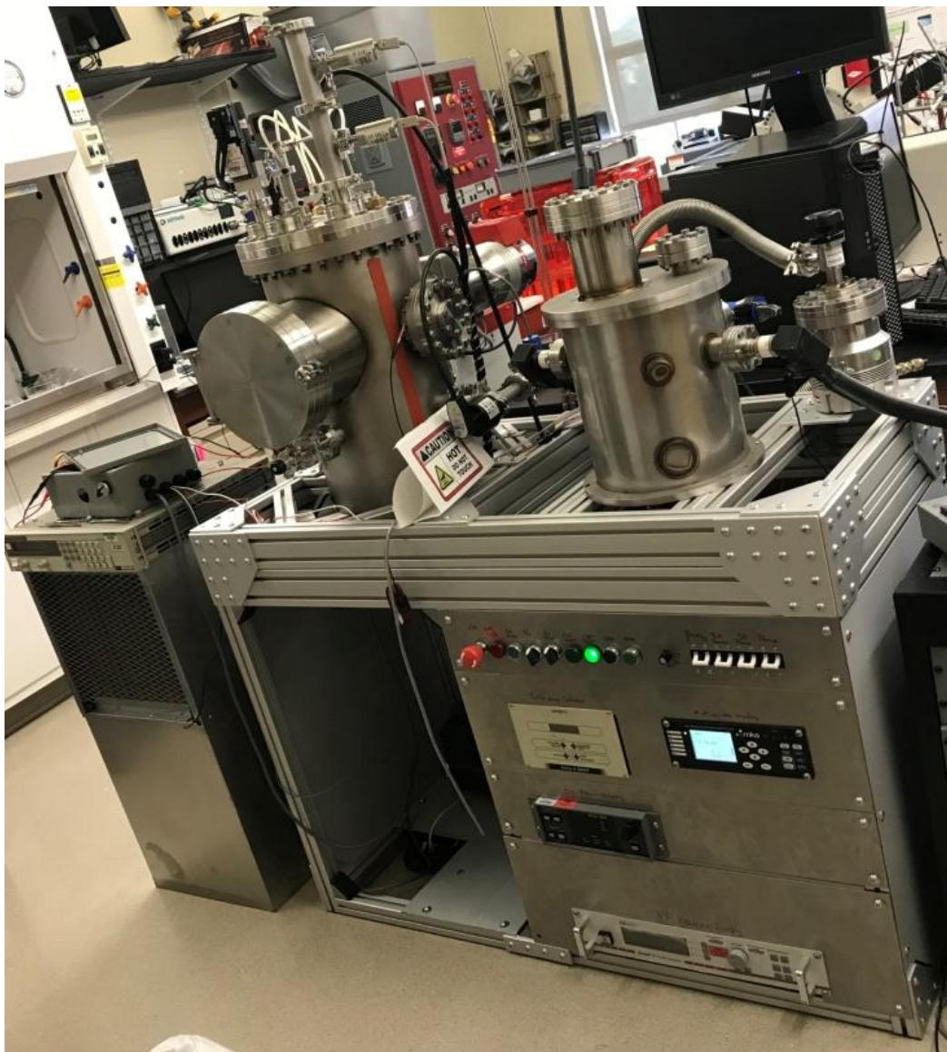
Fig. 12 RF / DC Magnetron system used for sputter deposition of the films.
