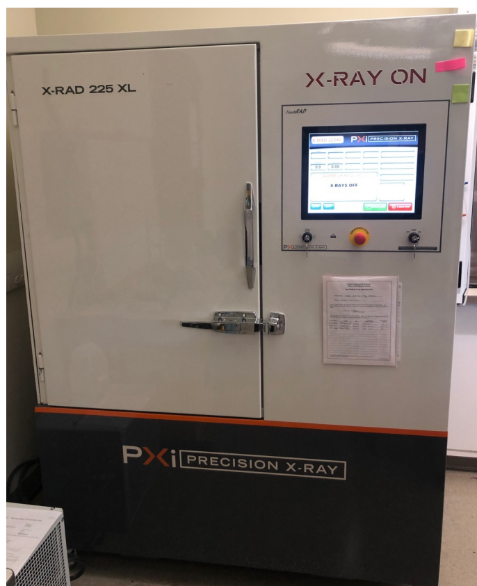
Figure 6.) The X-RAD 225 XL irradiator used for the experimental procedures.
