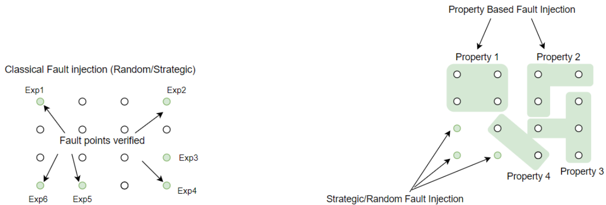
Figure 53: Classical Fault Injection vs Property Based Fault Injection
