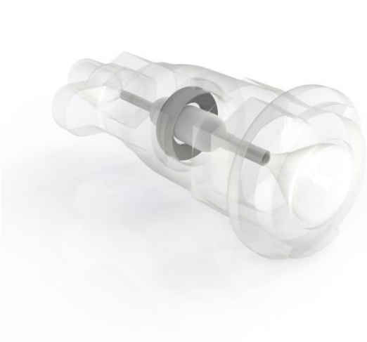
Figure 5.2: Overview of device geometry showing (a) CAD rendering with inlet and outlet connections, stainless steel capillaries, size 0 capsule, and rubber O-ring, and (b) internal flow pathway used for the CFD domain.
