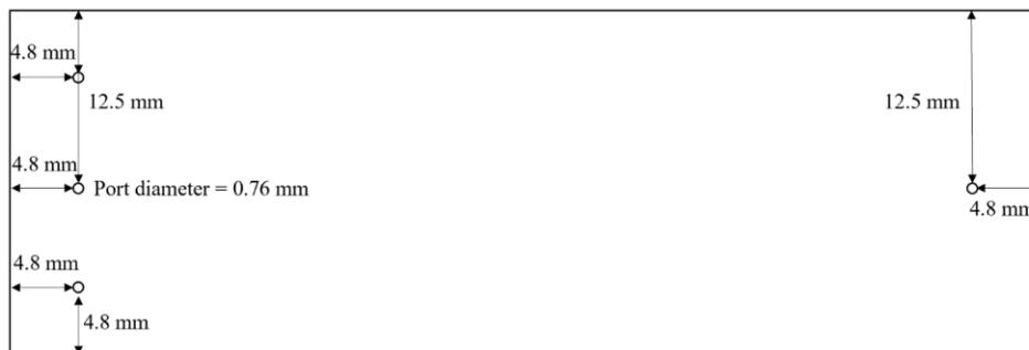
Figure 36 – Port placement of microdrilled holes in standard glass slide for the ‘bottom’ of the microfluidic reactor assembly.
