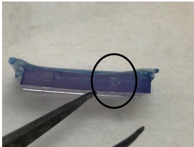
Figure 4.25 Cross-sectional view of modified systematic leak testing of NC representing no introduction of fluid into the well structure.
