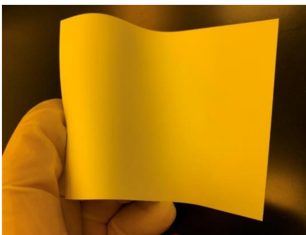
Figure 2.1 NC membrane. 7.9 cm x 10.5 cm with 0.2 \mu\text{m} pore size. Manually flexed to visualize NC flexibility and semi-rigid behavior.
