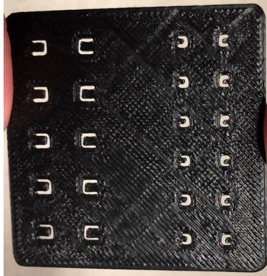
Figure 4.6 3D Printed shadowmask with U-Shaped filament pattern.
