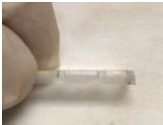
Figure 4.22 Realization of cross-sectional schematic as seen in Fig. 4.21 of modified PDMS well structures.
