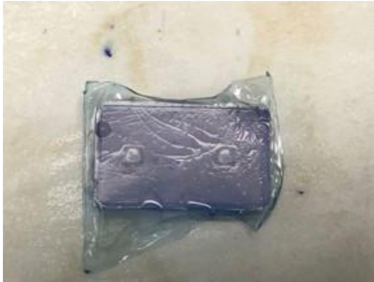
Figure 4.24 NC membrane atop PDMS well structures. Samples submerged in DI Water/Toluidine Blue fluid mixture for 1.5 months for leak testing at time of publication.
