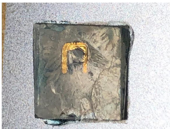
Figure 4.18 NC membrane over PDMS well structure with Blue Toluidine dye placed in well structure. Well structure, dye, and NC membrane glued to Si substrate. Submerged in DI water for 3 hours for initial testing.
