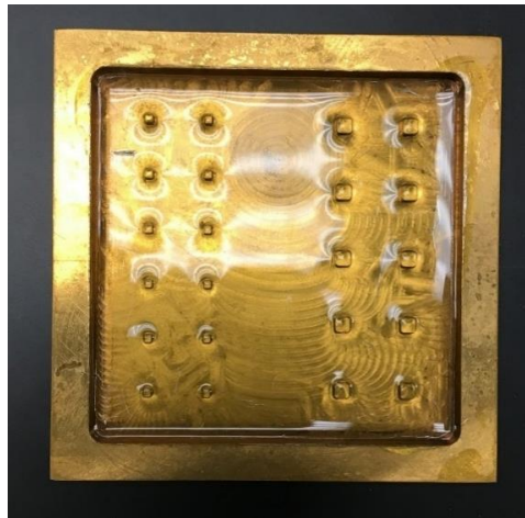
Figure 3.2 Aluminum plate (50 cm x 50 cm x 0.8 cm) machined to create a mold for casting PDMS well structures. Titanium Nitride (TiN) has been deposited on the surface of the aluminum via Atomic Layer Deposition (ALD) to create a low adhesion surface to assist the removal of cured PDMS Well structures. Using 3 g of PDMS base and 0.3 g of PDMS curing agent produces well structures with a depth of 1.5 mm.
