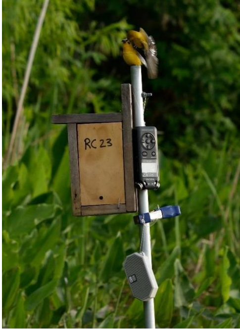
Figure 2. Staged Nest Intruder set-up in the field. A Tascam DR-05 recorder and Altec Lansing Mini H20 2 Bluetooth Speaker are looped around the nest box pole.
