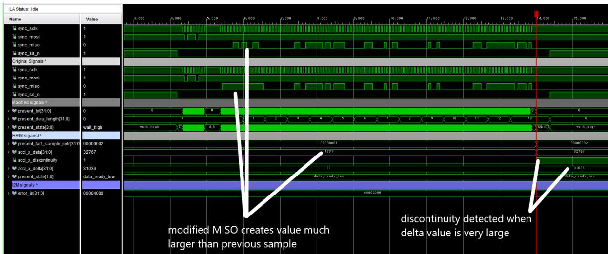
Figure 5.20 Discontinuity Fault Injection Results
