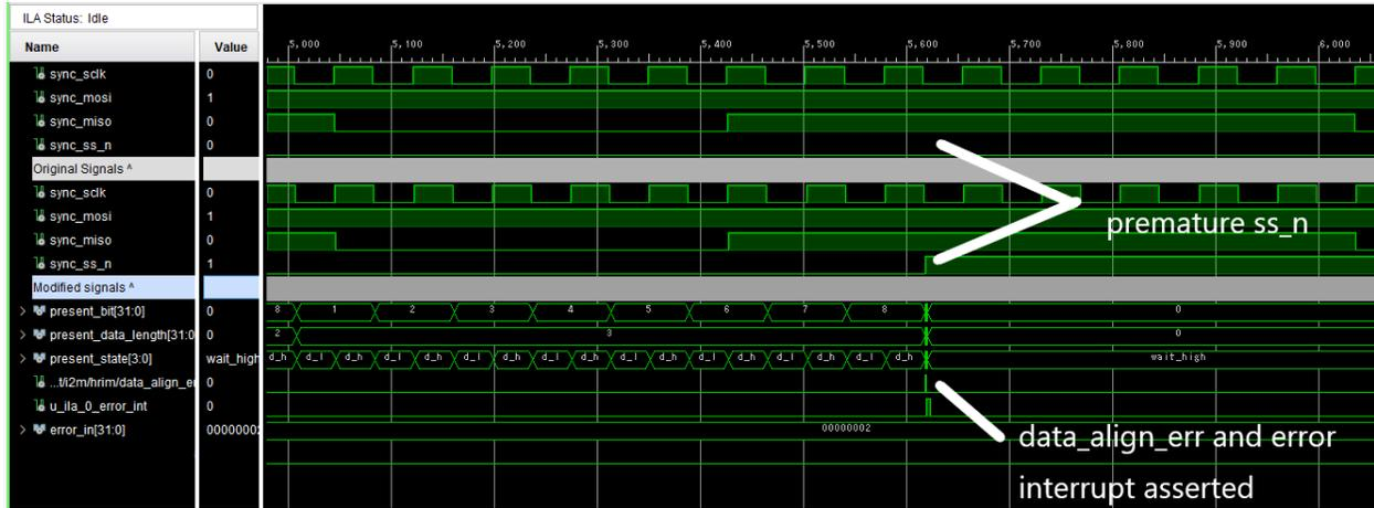
Figure 5.10 Data Alignment Fault Injection
