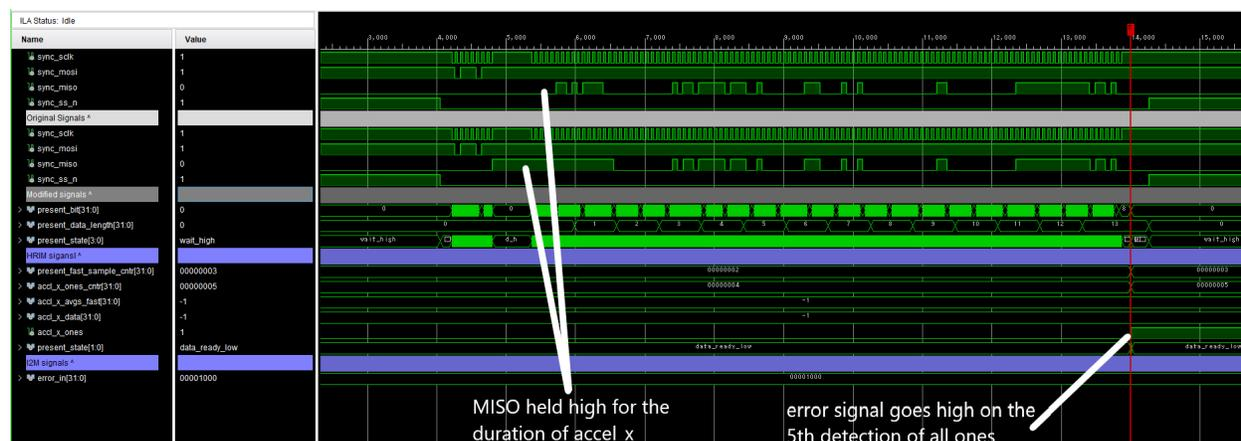
Figure 5.18 Stuck-At Ones Fault Injection Results
