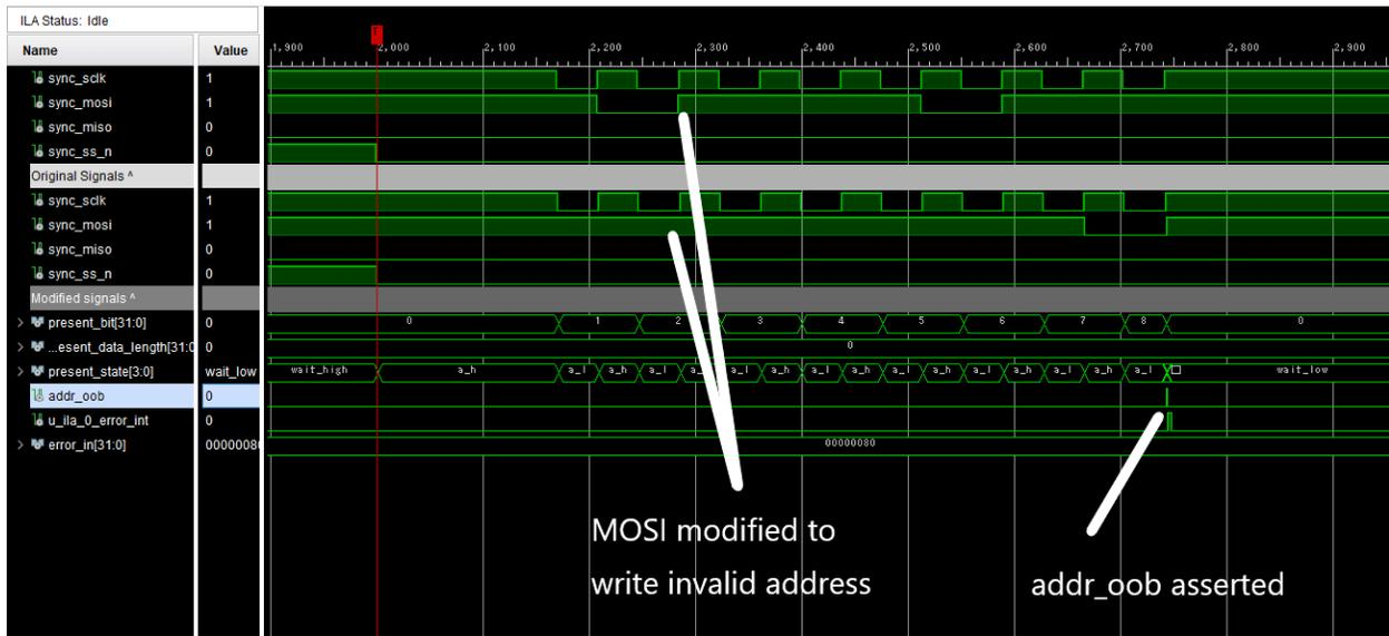
**Figure 5.9** Invalid Address Fault Injection
