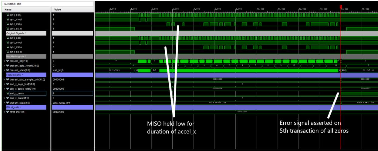
Figure 5.19 Stuck-At Zeros Fault Injection Results
