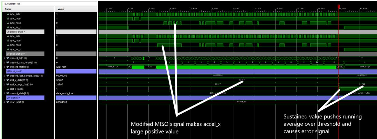
**Figure 5.21** Range Fault Injection Results
