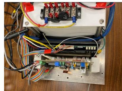
Figure 11: Controller/Power Assembly rear view
