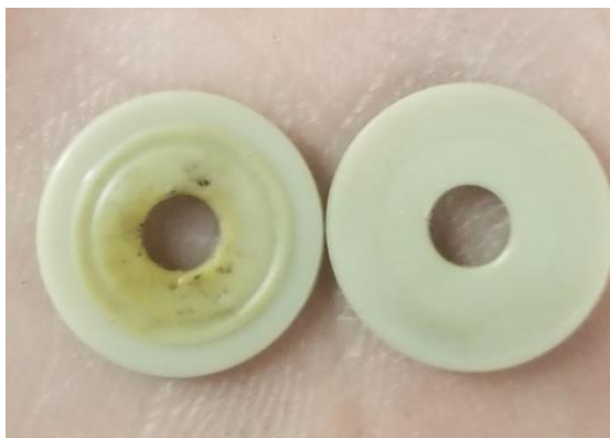
Figure 2511 Burned out regulator seals from the back pressure regulator
