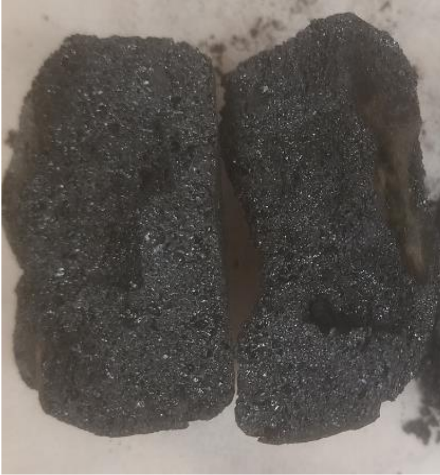
Figure 29. Photograph of a cleaned coal that has fused due to high temperature.
