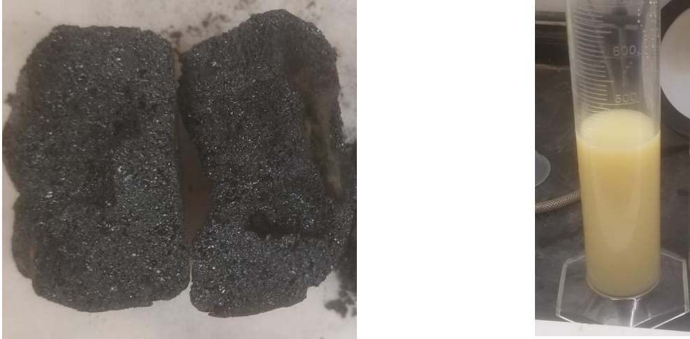
Figure 36. Products from experiment E102219: coal (left) and dissolved minerals (right)
