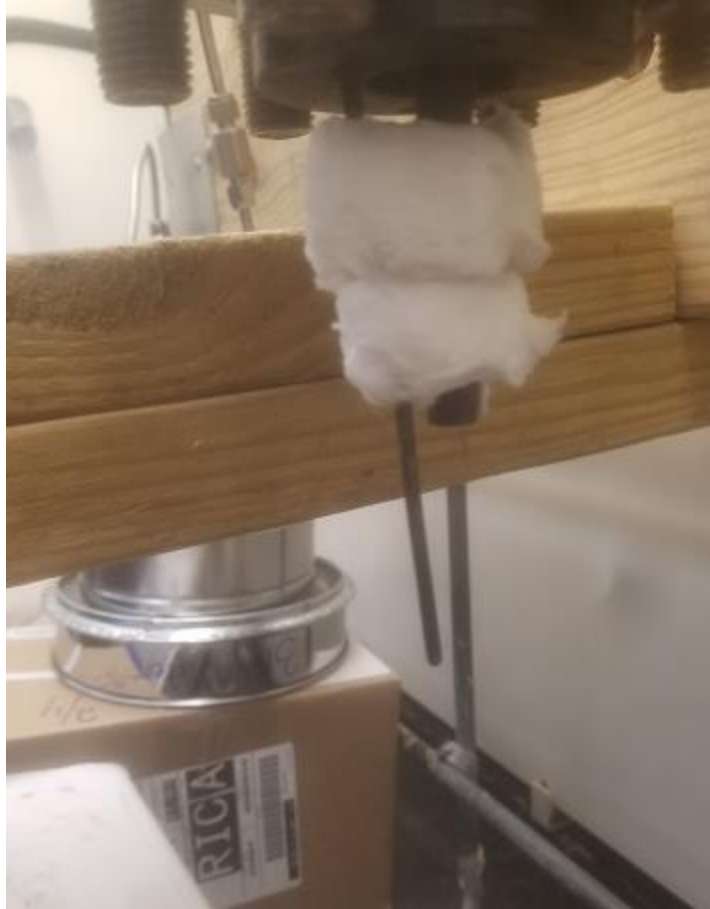
Figure 26. Photograph showing thermos-well containing thermocouple.
