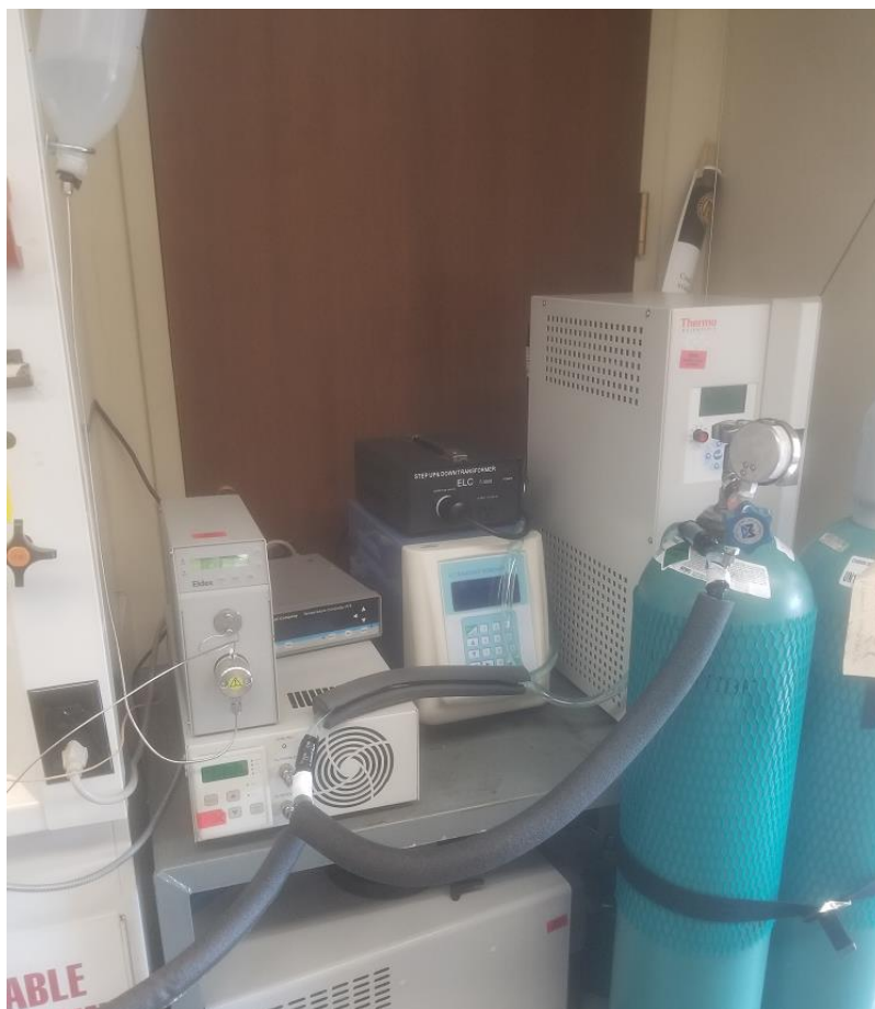
Figure 18. Photographs of the CO 2 and H 2 O pumps
