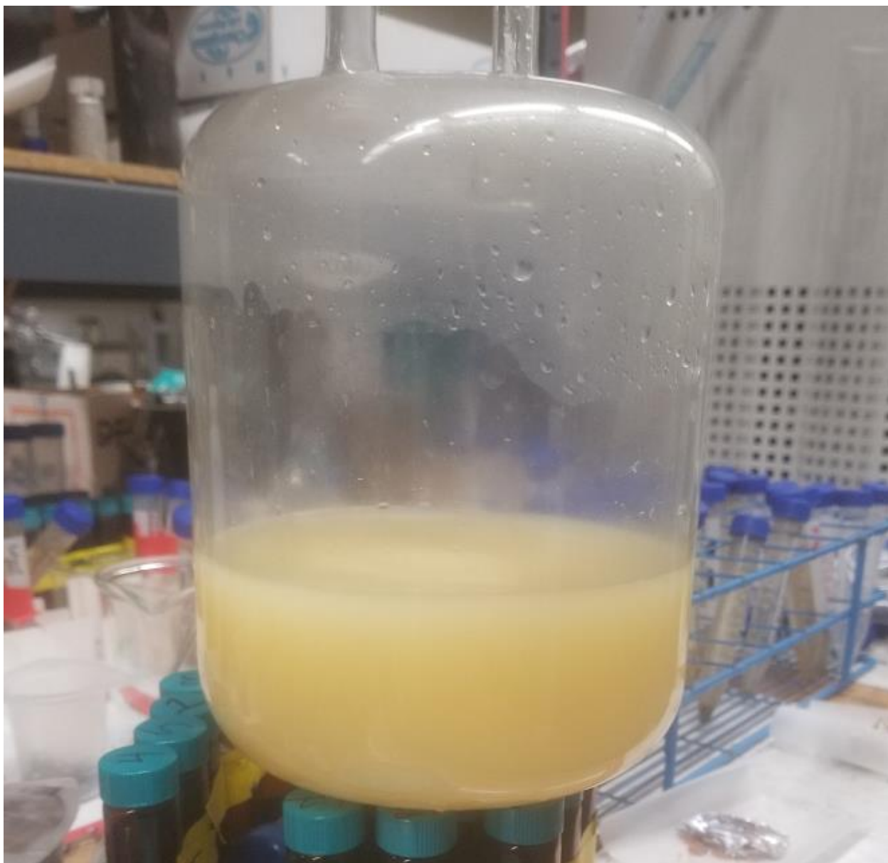
Figure 30. Outlet aqueous stream containing extracted material.
