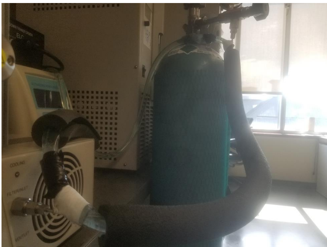
Figure 24. Photograph of the cooling heat exchanger to liquefy CO 2 .
