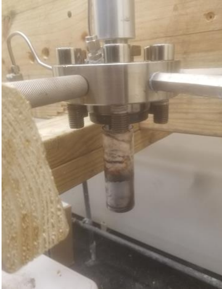
Figure 27. Photograph of glass containment vessel stuck to the vessel
