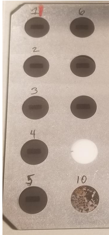
Figure 32. Photograph showing coal pellet that have gone through laser ablation test.
