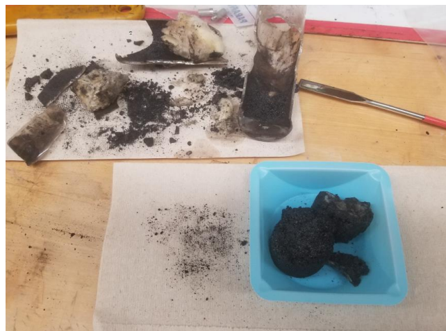
Figure 28. Photograph of the broken glass containment vessel.
