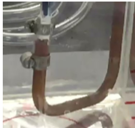
Figure 2.2: U bend in copper tube
