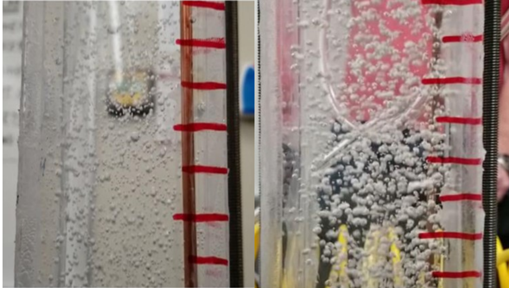
Figure 3.1: Bubbly Flow (L and R), red lines indicate \frac{1}{2} " ( \sim 12.7\text{mm} ) increase in height
