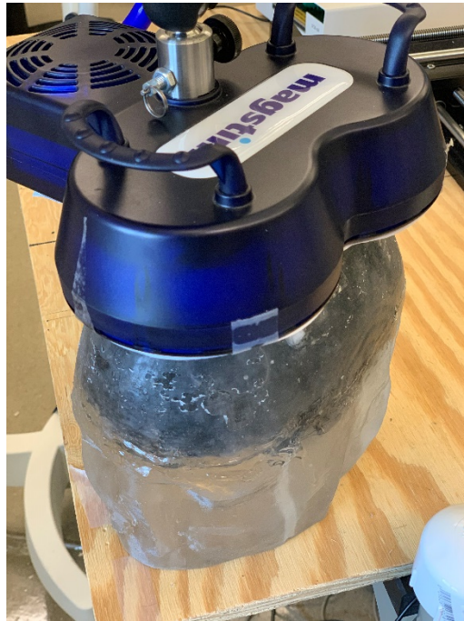
Figure 55 Experimental set-up where time-varying magnetic field by the transcranial magnetic stimulator is applied on the physical head phantom.
