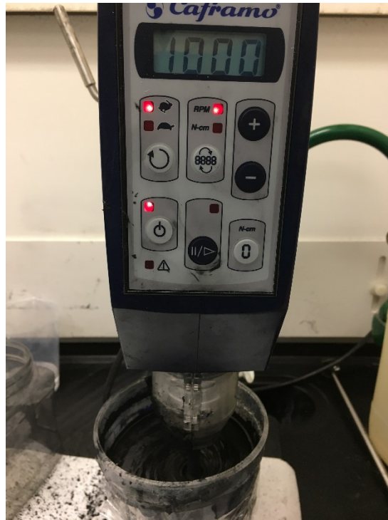
Figure 24 The MWCNT is added to the PDMS base and mixed with the mechanical stirrer at 1000 rpm
