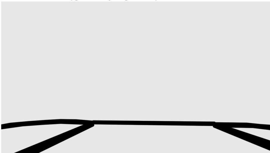
FIGURE 4.10: Segmentation of the ZED camera image, where black pixels are pixels which view the aircraft's body rather than the surrounding environment, and thus are unusable for the intended sensing operations. Note that under indoor lighting conditions, the propellers are not visible in flight and do not obscure the camera.
