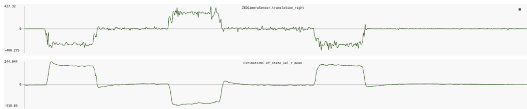
FIGURE 4.11: Periods of constant-velocity movement, showing the raw vs. estimated state. The estimated state has removed much of the noise from the input signal, but displays a slight overshoot behavior after sudden accelerations. The flipped signal polarity is a side-effect of the output being in a difference reference frame from the input.
