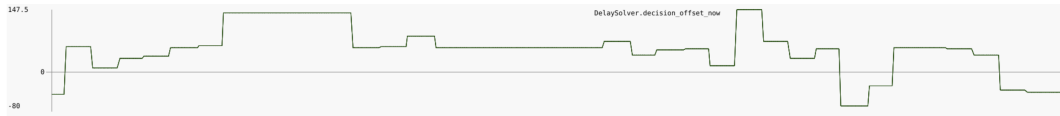
FIGURE 4.8: Delay Solver "decisions" over time, showing a lack of agreement on any single value. Values are in milliseconds.
