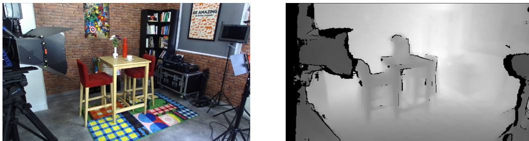
FIGURE 3.12: Sample Image output of the ZED Camera: RGB and Depth (visualized as Greyscale)
