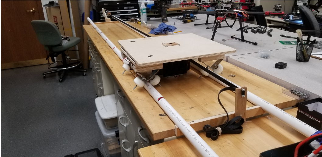
FIGURE 4.2: The "sled" created for use as a known motion source.
