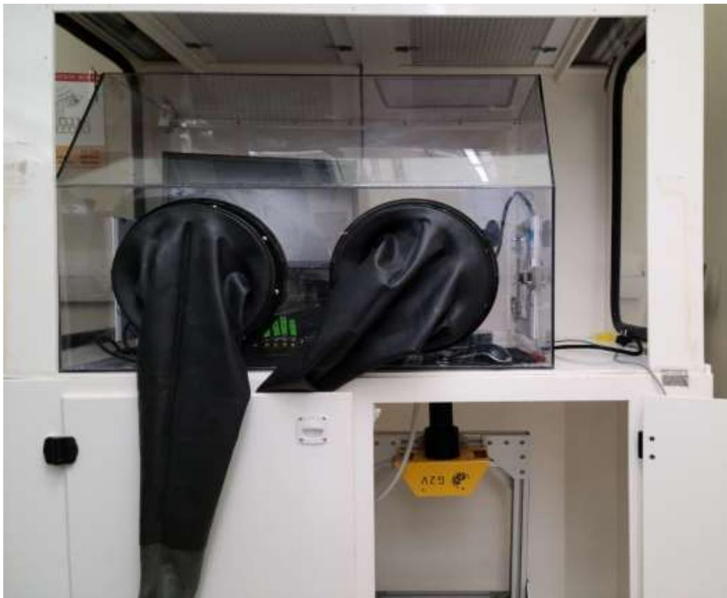
Figure 5.2: Setup of Glovebox + Solar I-V System for characterizing  $\text{CH}_3\text{NH}_3\text{PbI}_3$  perovskite solar cells
