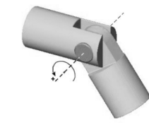
Fig. 30. Revolute joint: one degree of freedom.
