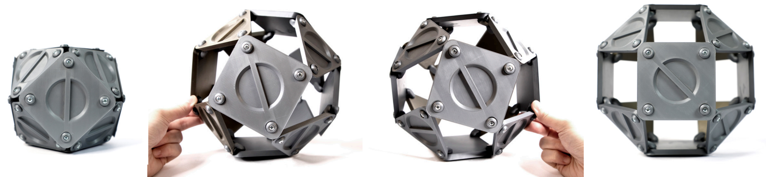
Fig. 36. The transformation of the polyhedral models can be actuated by moving a single polygonal face.
