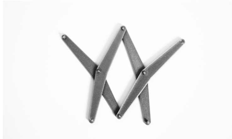
Fig. 21. Angulated scissors mechanism capable of two-dimensional expansion.
