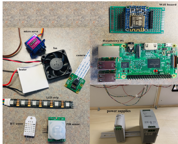
Figure 3.11: Picture of sensors, actuators, sources, and control boards used in the smart building
