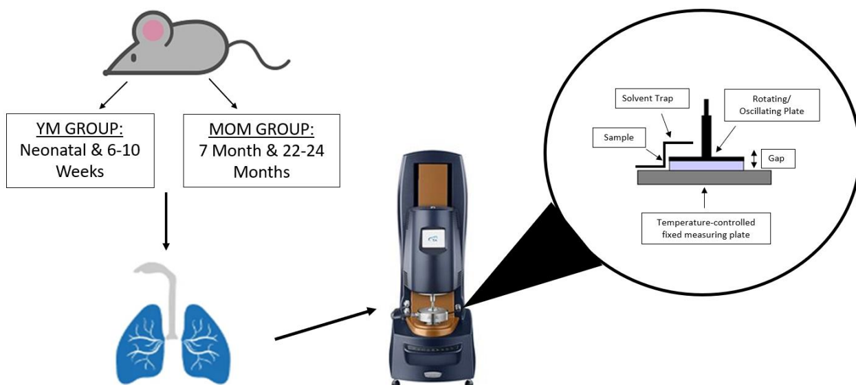
Figure 9. Schematic of protocol set up for rheological testing.
