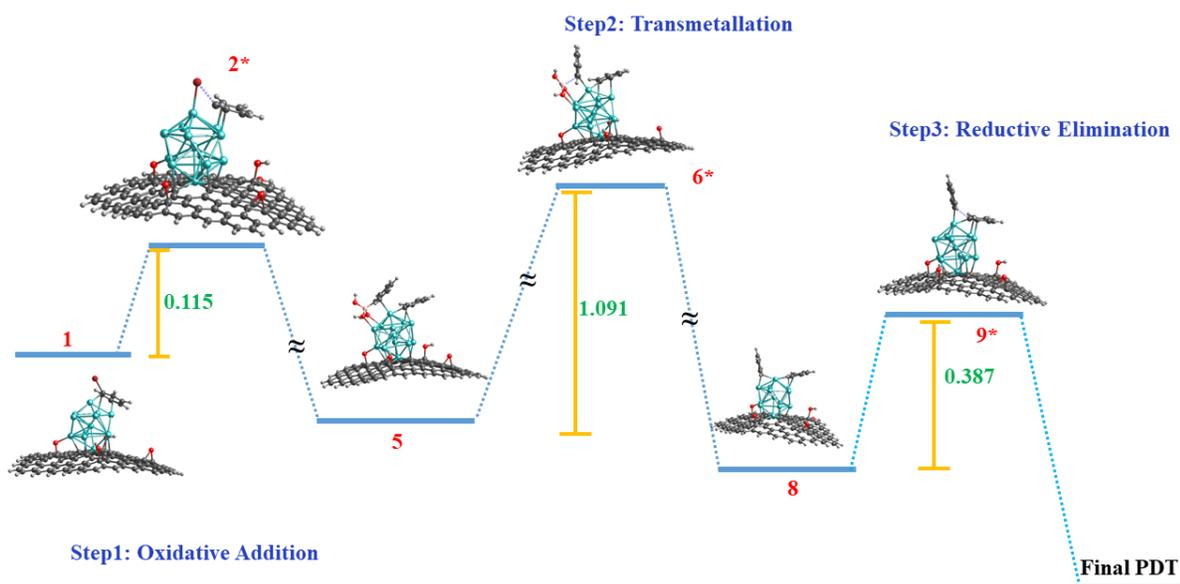
Figure 6.9 Reaction Pathway for the interacting system in case of Pd<sub>13</sub> on RGO support.
