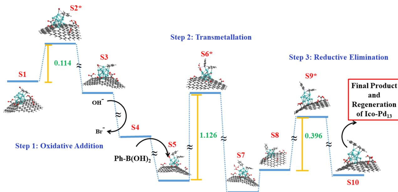
Figure 6.8 Reaction Pathway for the non-interacting system in case of Pd<sub>13</sub> on GA Support.
