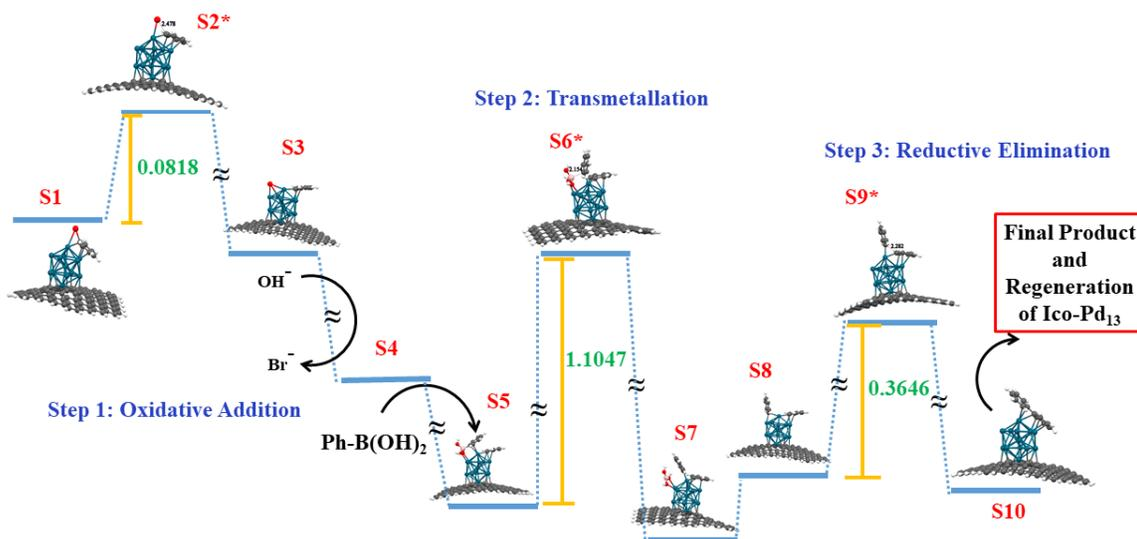
Figure 6.6 Reaction Pathway for the non-interacting system in case of Pd<sub>13</sub> on defected Graphene Support.
