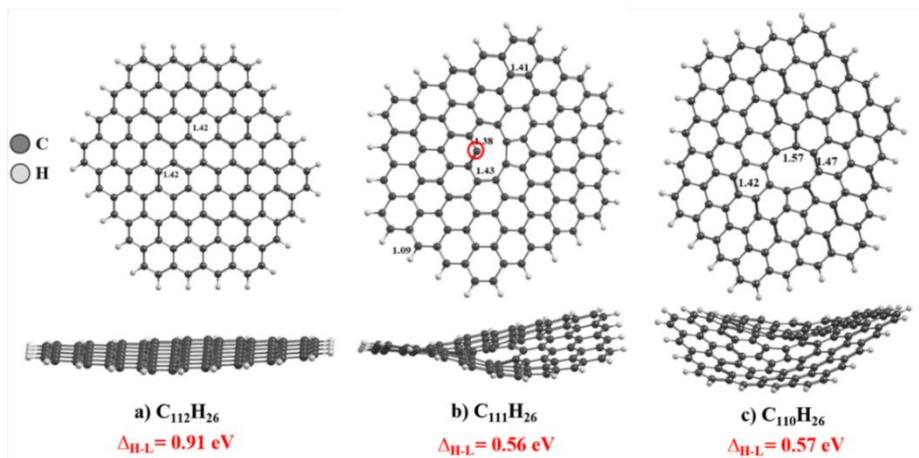
Figure 6.4. Optimized (ADF:PBE/TZ2P) geometries of a) pristine ( $C_{112}H_{26}$ ) b) single C vacancy ( $C_{111}H_{26}$ ) and (c) double C vacancy ( $C_{110}H_{26}$ ) graphene sheets. The calculated HOMO–LUMO gaps ( $\Delta_{H-L}$ ) and important bond lengths (Å) are also included.
