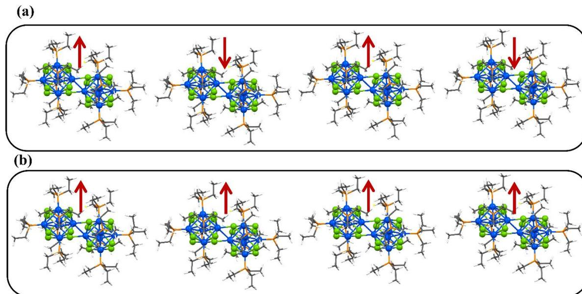
Figure A1 Schematic showing (a) antiferromagnetic-coupling between dimers in the cluster assembled solid  $\{[\text{Co}_6\text{Se}_8(\text{PEt}_3)_5]_2(\text{Toluene})_2\text{C}_{140}\}_2$  (b) ferromagnetic-coupling between dimers in the solid. The red arrows show the direction of the spin-magnetic moment at the junction of the dimer. The antiferromagnetic coupling is more stable than ferromagnetic coupling by only 0.03 eV.
