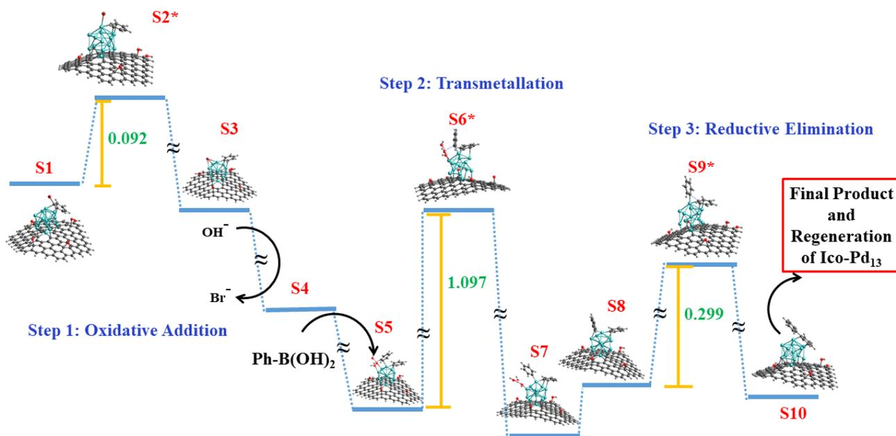
Figure 6.7 Reaction Pathway for the non-interacting system in case of Pd<sub>13</sub> on RGO support.
