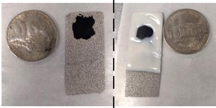
**Figure A1.1.** [Left] nickel foam with electrode ink and reference object (U.S. nickel) prior to templating and [Right] the electrode and reference object post templating.
