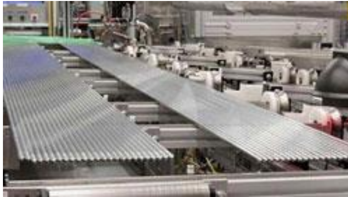
Figure 1.2 Coated Zircaloy ATF Cladding [16]
