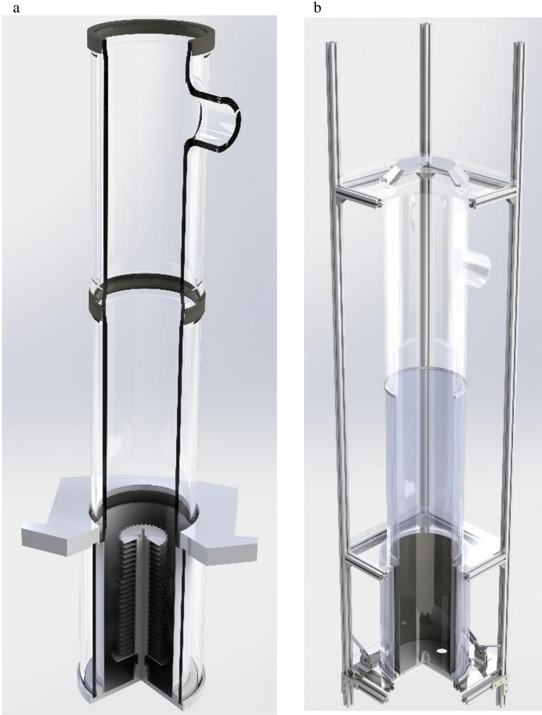
Figure 9.2: Cutaway views of (a) the Buchi Nano Spray Dryer B-90 tower and (b) the VCU Small Particle Spray Dryer tower with frame.
