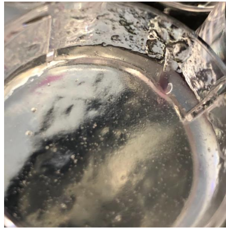
Figure 22: 2% (w/v) alginate hydrogel printed into gelatin slurry with \text{CaCl}_2 concentration of 100 mM. The pink-colored components indicate alginate hydrogel deposits from the extrusion process.
