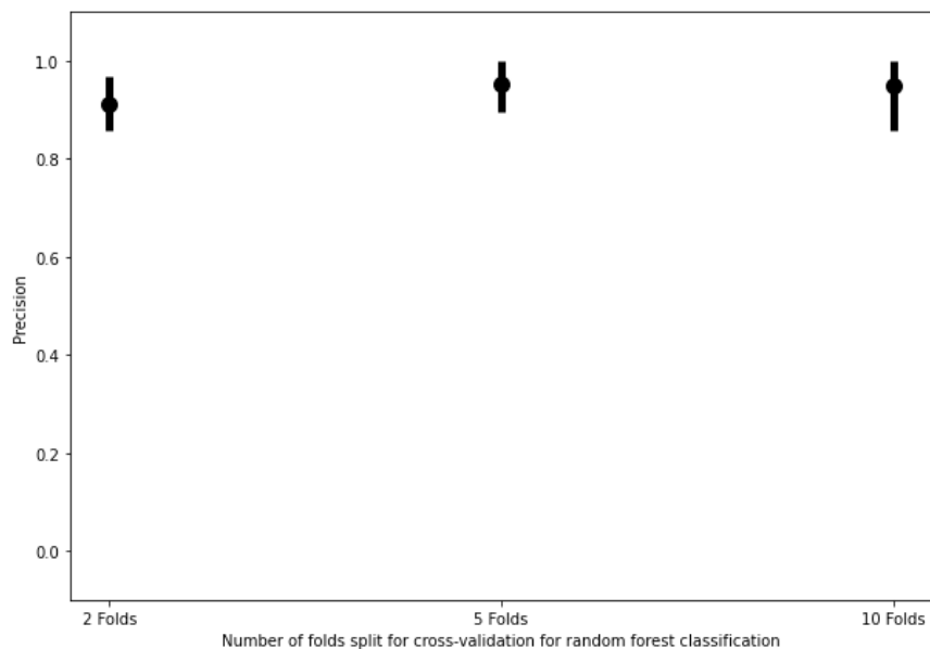
Figure S26. Precision scores of filament diameter classification models based on the number of folds tested for random forest regression models. The upper and lower bounds of the error plots represent the maximum and minimum precision produced for each fold division.
