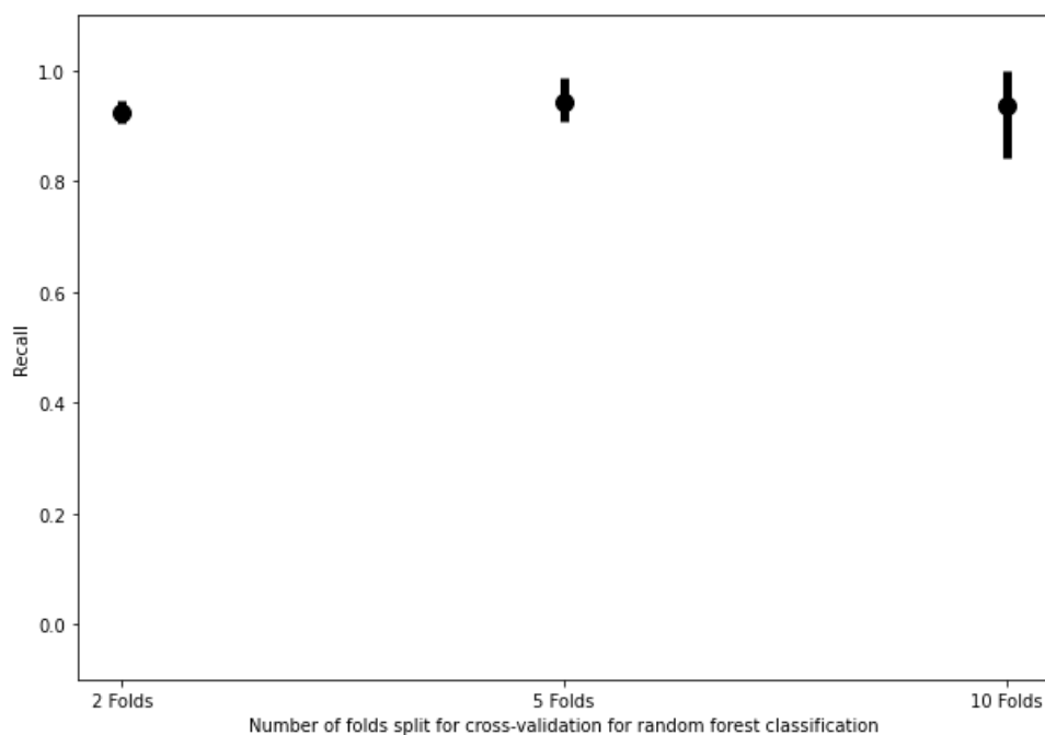
Figure S19. Recall performance of the random forest classification cell viability model on different k-fold cross validation tests. The upper and lower bounds of the error plots represent the maximum and minimum metric values produced for each fold division.
