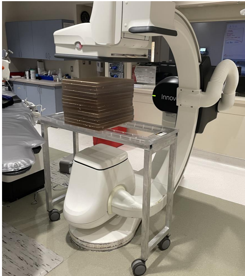
Figure 2: Shows the setup of the study with 14 inches of PMMA on top of the cutout in the correction location over the x-ray tube with the patient table removed.
