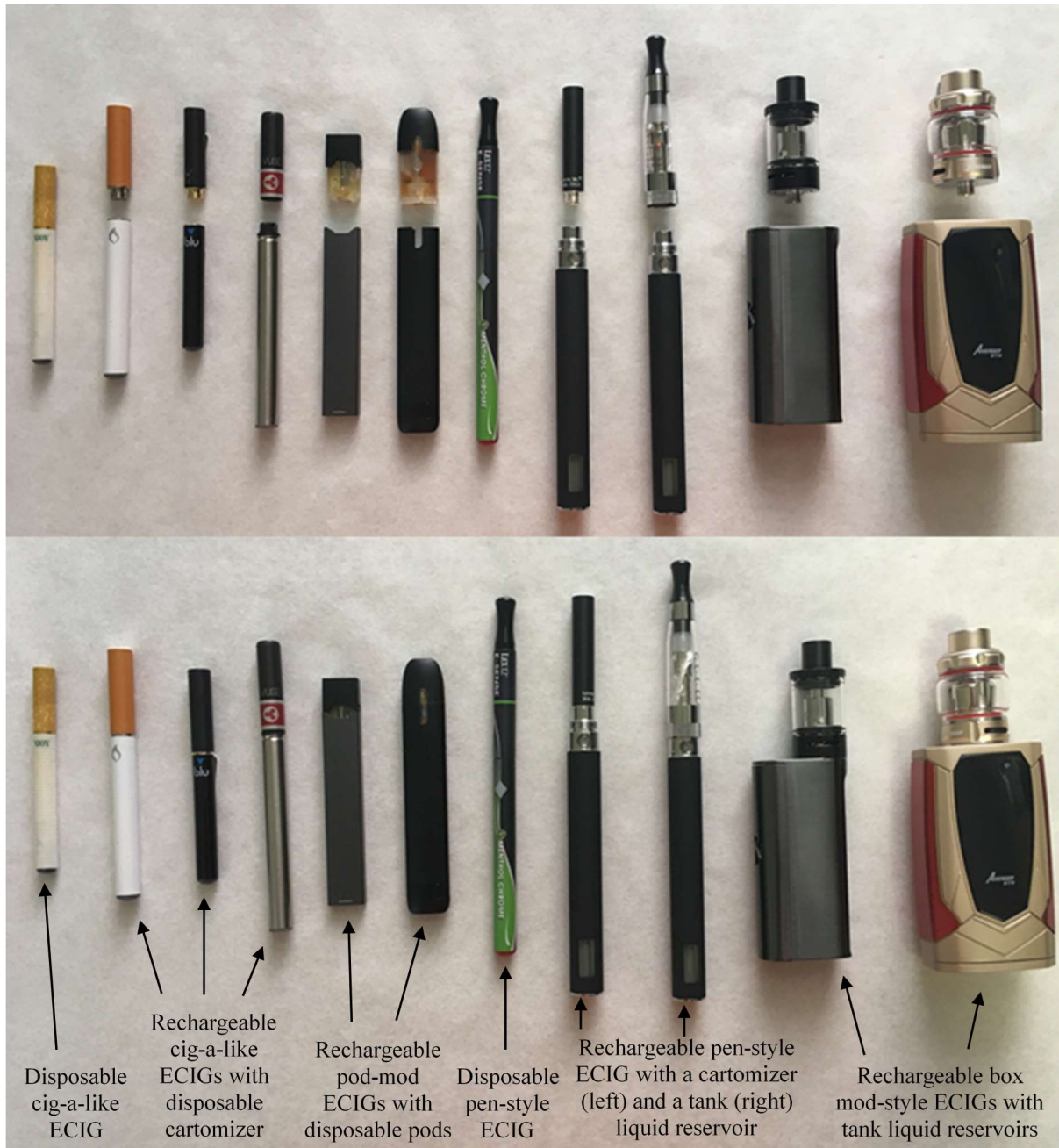
Figure 1. Various ECIG styles and devices. The top image displays the liquid reservoirs detached from the battery component and the bottom picture displays the device attached to the liquid reservoirs.
