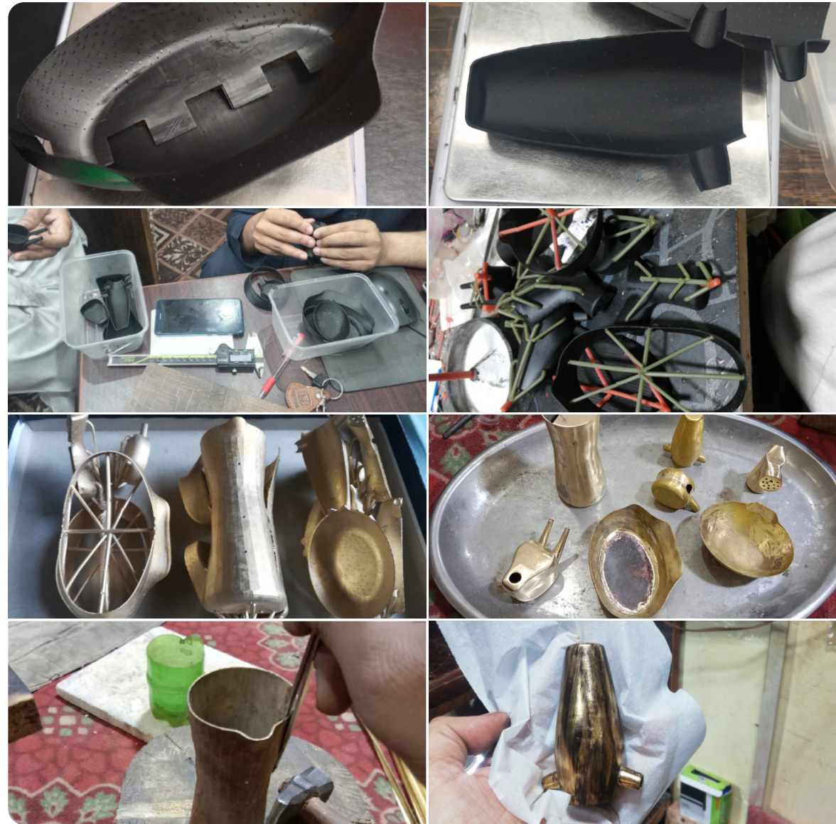
Figure 45: Lost-wax casting process in Pakistan
