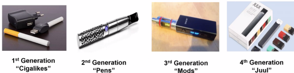
Figure 1.1. Common ECIG Devices Showing the Evolution from First Generation (Cig-A-Likes) to Fourth Generation Cartridge Devices (JUUL).
