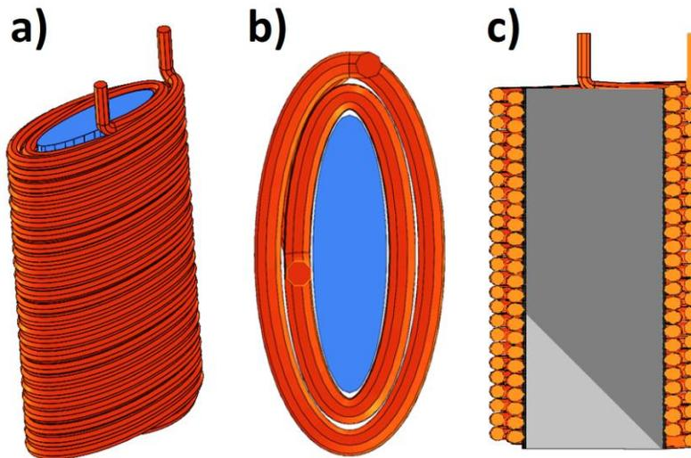
Figure 45 – Dual solenoid of elliptical shape with AISI 1010 carbon steel core. a) Isometric view; b) top view c) internal view (V-shape profile in dark gray and complement for flat profile in light gray).
