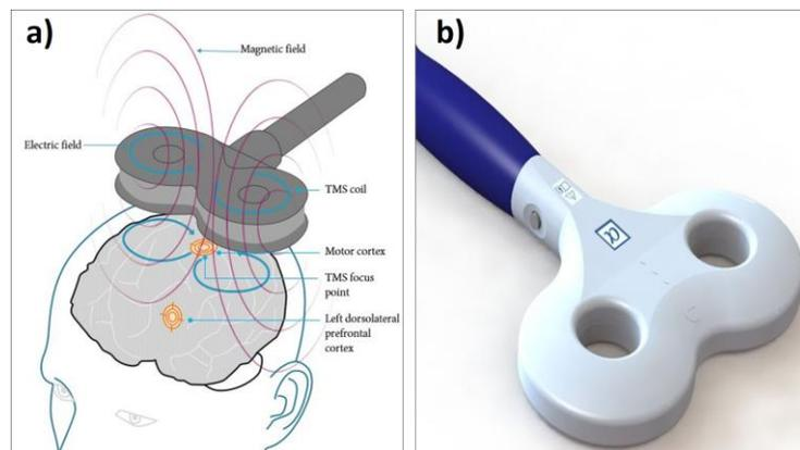
Figure 1 – a) Illustration of transcranial magnetic stimulation using a figure-of-eight coil. Notice how the magnetic field lines penetrate the different layers of the human head to induce an electric field of a circular shape whose intensity is higher toward the center. Source: [9]. b) Commercial figure-of-eight coil, model D70 Alpha Flat of the manufactured MAGSTIM, used in clinical settings [10].
