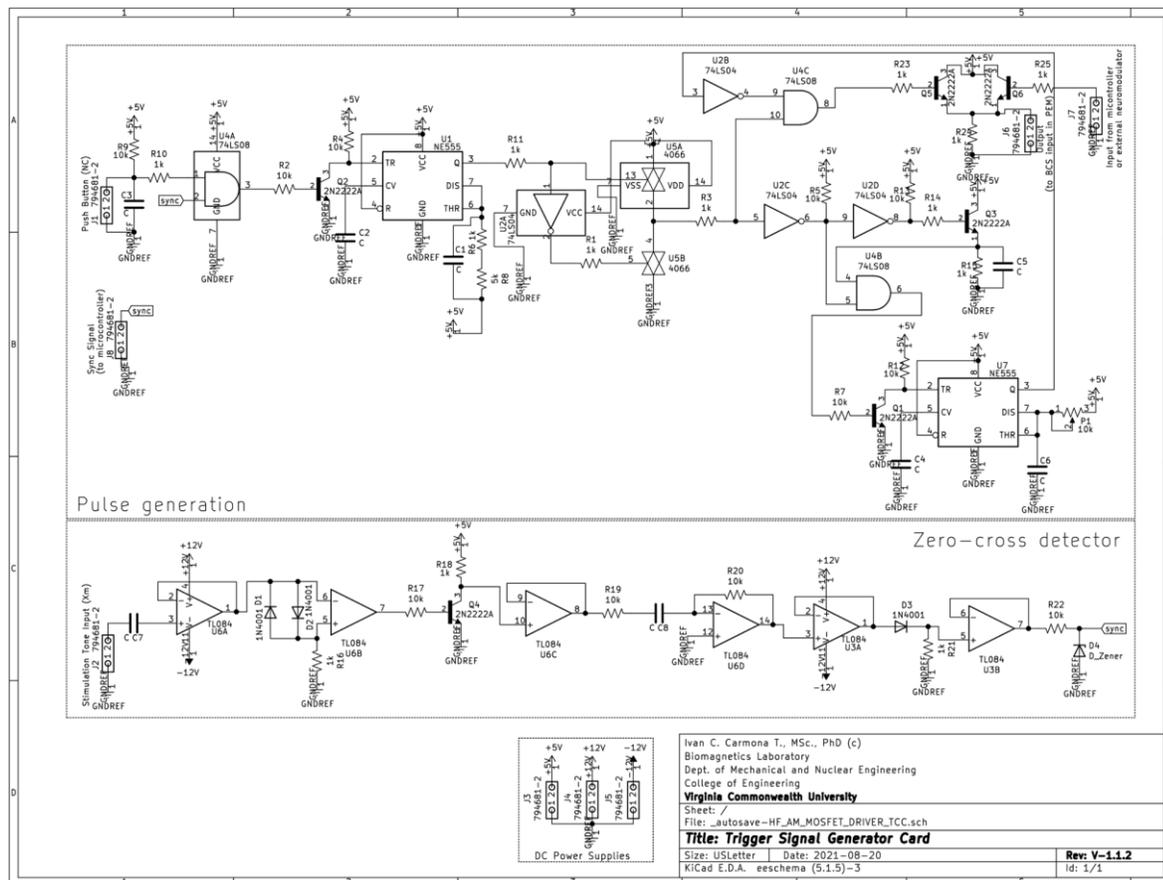
Figure 35 – Circuit diagram of the Trigger Signal Generator Card. The input signal may originate from the push button (J1) in phase with the referential stimulating tone (J2) or from an external equipment through the input J7.
