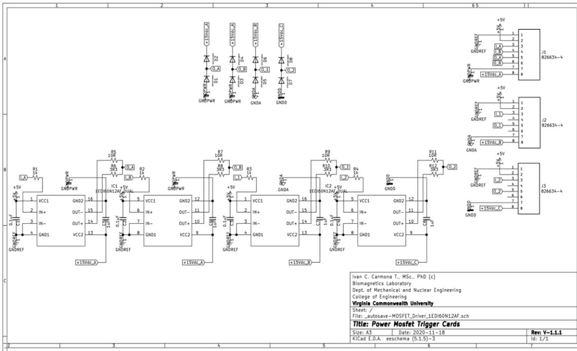
Figure 34 – Circuit diagram of the *power MOSFET trigger cards*. The card has been designed to be pin-compatible with the output of PEM. The clamping diodes in the upper part help to stabilize the voltage in the gate that may course overcurrent in each of the drivers.
