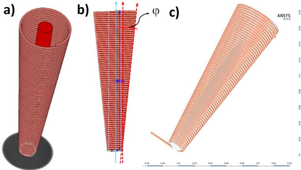
Figure 42 – Simulated conical coil with MnZn ferrite core. a) isometric view. b) Front view with opening angle. c) Isometric view of the coil with a core with 120° of tip sharpening.
