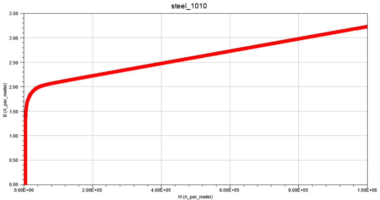
Figure 29 – B-H curve for AISI 1010 carbon steel, showing a linear region of fixed slope in the beginning, and then a saturation point at approximately 2 T.
