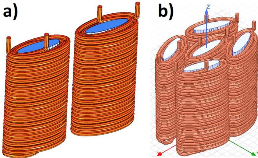
Figure 47 – Double array of elliptical dual solenoids (AISI 1010 carbon steel or air core in blue). b) Final quintuple array of dual solenoids.
