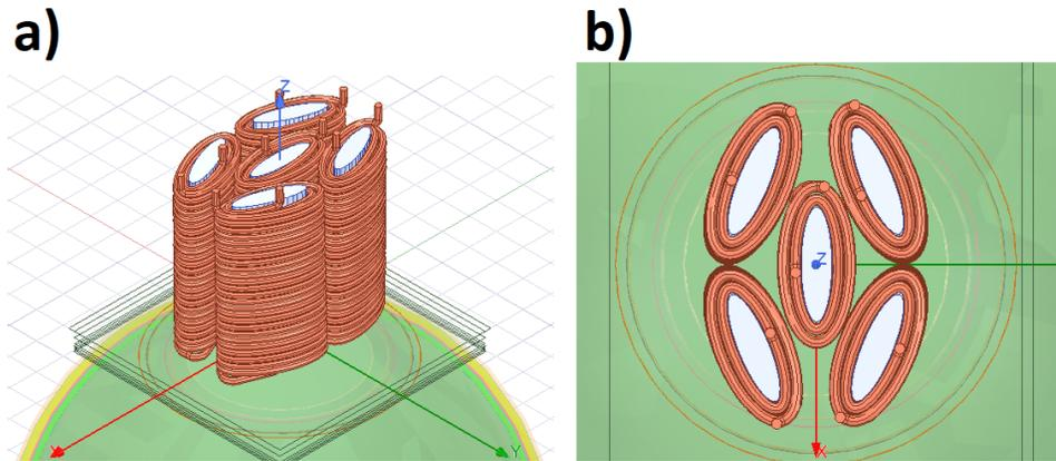
Figure 61 – Quintuple arrangement of elliptical solenoids and planes. a) Isometric view. b) Top view.
