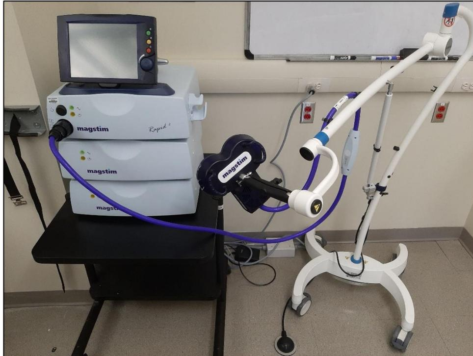
Figure 4 – Photograph of the commercial TMS stimulator, model *Rapid 2* of the manufacturer *MAGSTIM*, used for experimentation at the Biomagnetics Laboratory, Virginia Commonwealth University. Notice the figure-of-eight coil connected to it and the relatively big size of the stimulator. This size is a consequence of the power electronics and heat dissipation system required to manage currents in the order of several kilo-amperes and voltages of several hundreds of volts.
