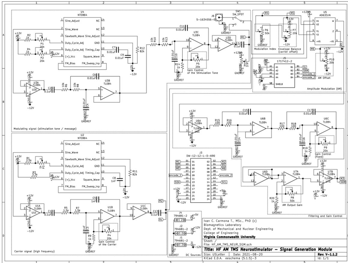
Figure 32 – Circuit diagram of the *signal generation module (SGM)*. Notice the presence of two signal generation modules whose outputs are preconditioned through operational amplifiers to be delivered to the mixer AD633JN. Then, the output is filtered and delivered to the *power electronic module (PEM)* in the point tagged as XAM.
