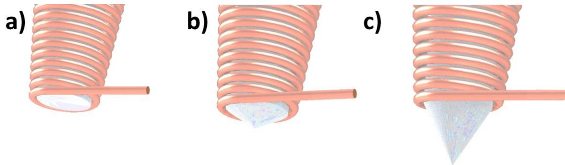
Figure 44 – Cases simulated for different degrees of tip sharpening in the core. a) 180 degrees (flat tip); b) 120 degrees; c) 60 degrees.
