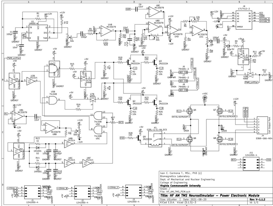
Figure 33 – Circuit diagram of the *power electronic module (PEM)*. The input identified as XAM comes from the SGM with the AM/DSB modulated signal. The input with the tag Xc brings the AM/DSB carrier to PEM to create the two-channel *dead time control signal*. J1, J2, and J3 are the output ports in which the trigger cards are connected.
