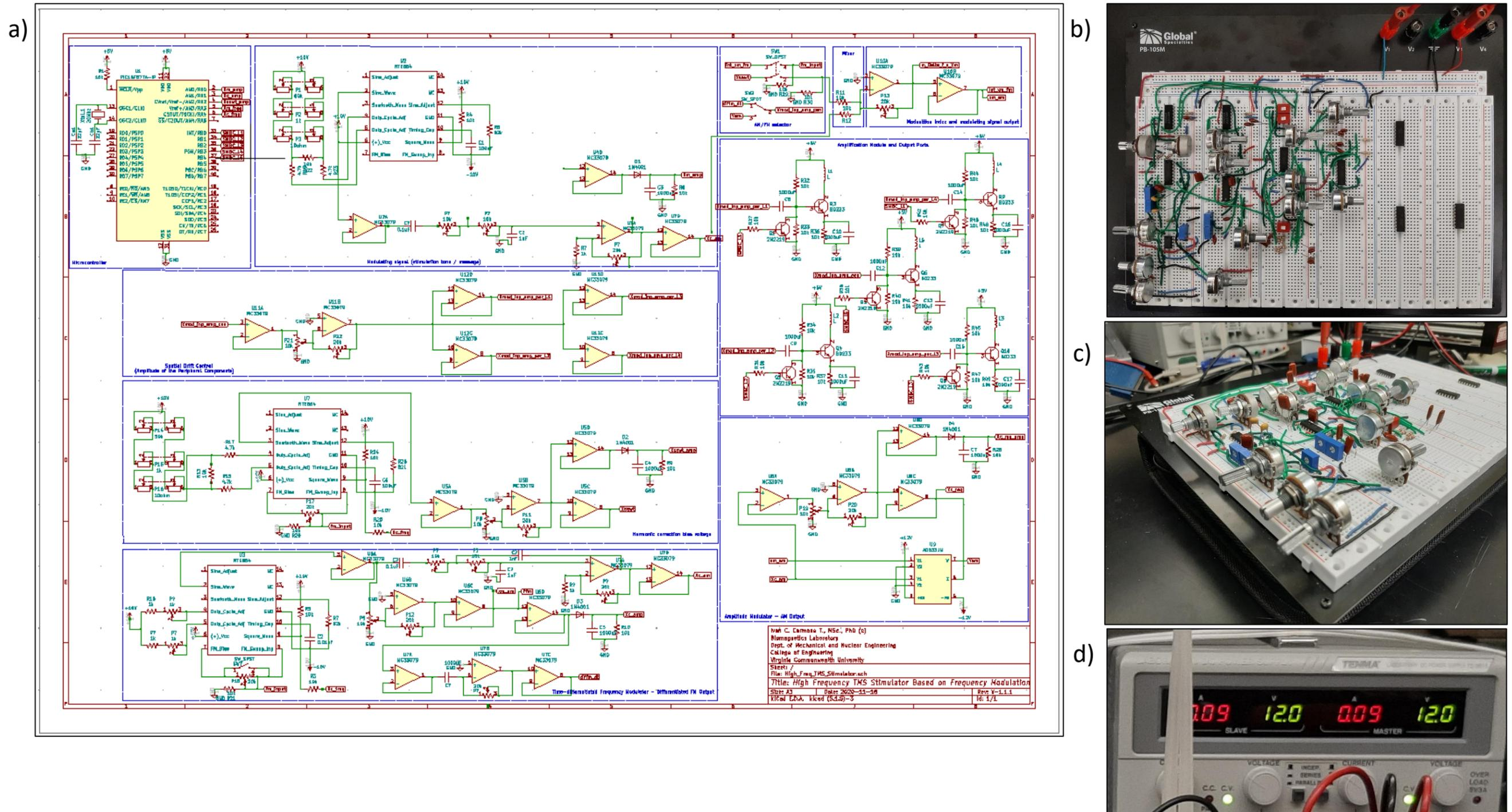
Figure 30– a) Circuit diagram of the designed high-frequency modulator based on AM (1<sup>st</sup> version). b-c) Circuit prototype built on a breadboard (front view (b) and isometric view (c)). d) Currents and voltages in the DC power source. At this stage, the circuit only needs the final stage of current amplification (coil terminals) to be completed.
