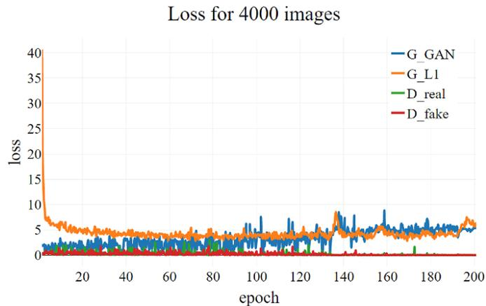
Figure 3.5: Loss curve for the model with 4000 training images.
