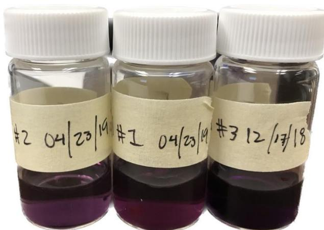
*Figure 37: Synthesized Ag nanoparticle solution showing stability. The prepared solutions are shown comparing their color from Purple to Burgundy to Violet from left to right. The solution on the right has shown stability for over four months at inside a refrigerator at the time of the photo.*
