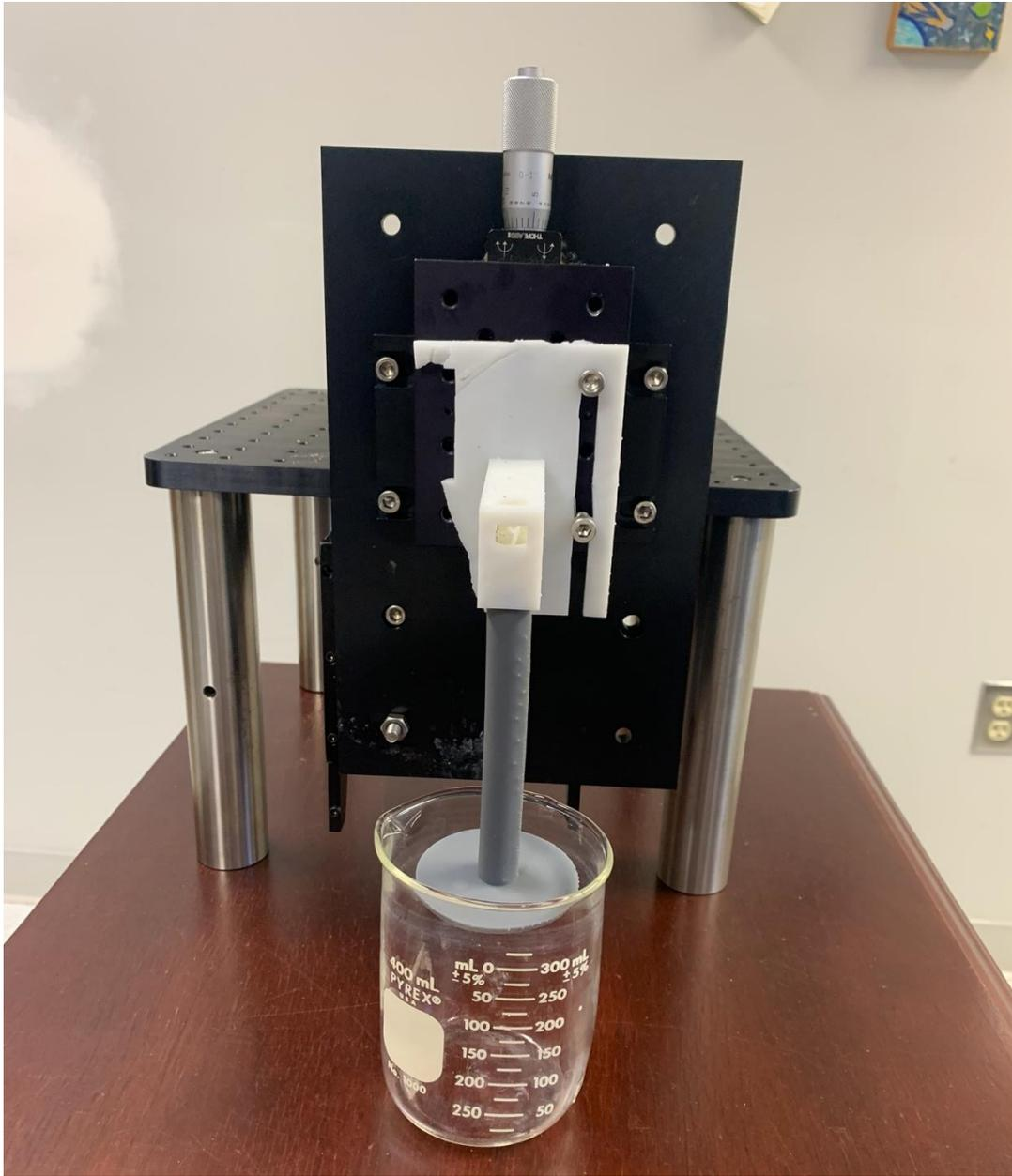
*Figure 41: QTF etching setup. The one-directional micrometer allows for the tips to be submerged into nitric acid at a controlled rate and at a stable depth. The tips were magnetically attached to the underside of the gray setup piece. The etching setup was a damaged early model and was thus sacrificial.*
