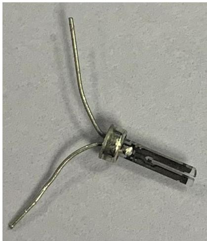
*Figure 33: De-Canned Quartz Tuning Fork. The quartz prongs have electrodes inside that are electrically isolated from one another. These electrodes are then connected to a metal leg.*
