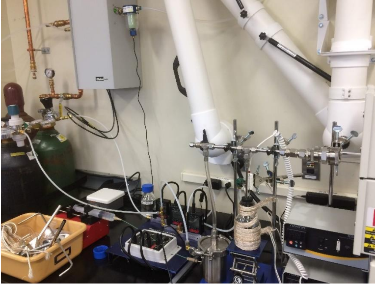
Figure 0-1. Part of the setup to generate aerosol flow before entering the furnace.
