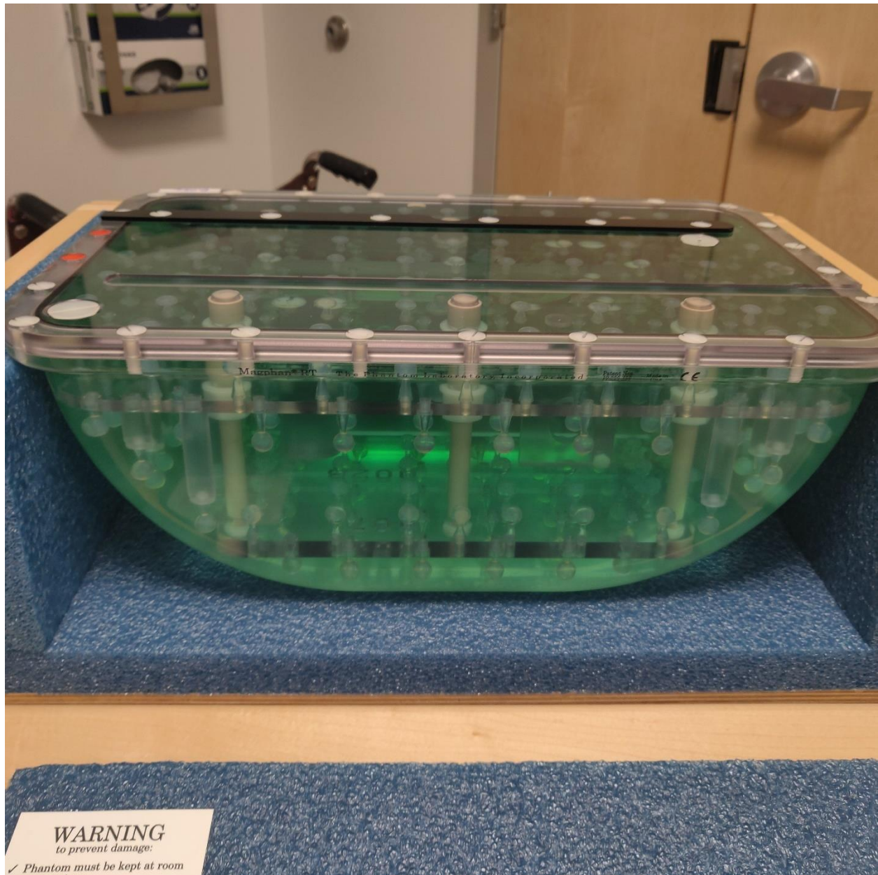
Figure 13. Photo of half of the MagPhan RT phantom in its storage container.
