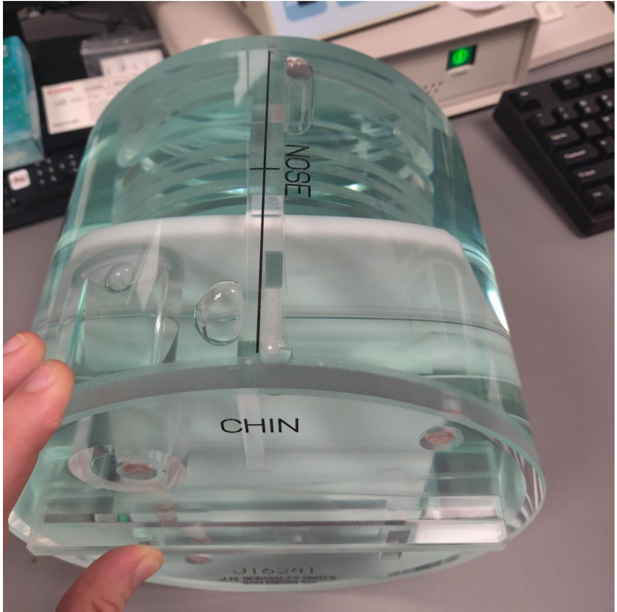
Figure 11. Photo of the large ACR MRI accreditation phantom.
