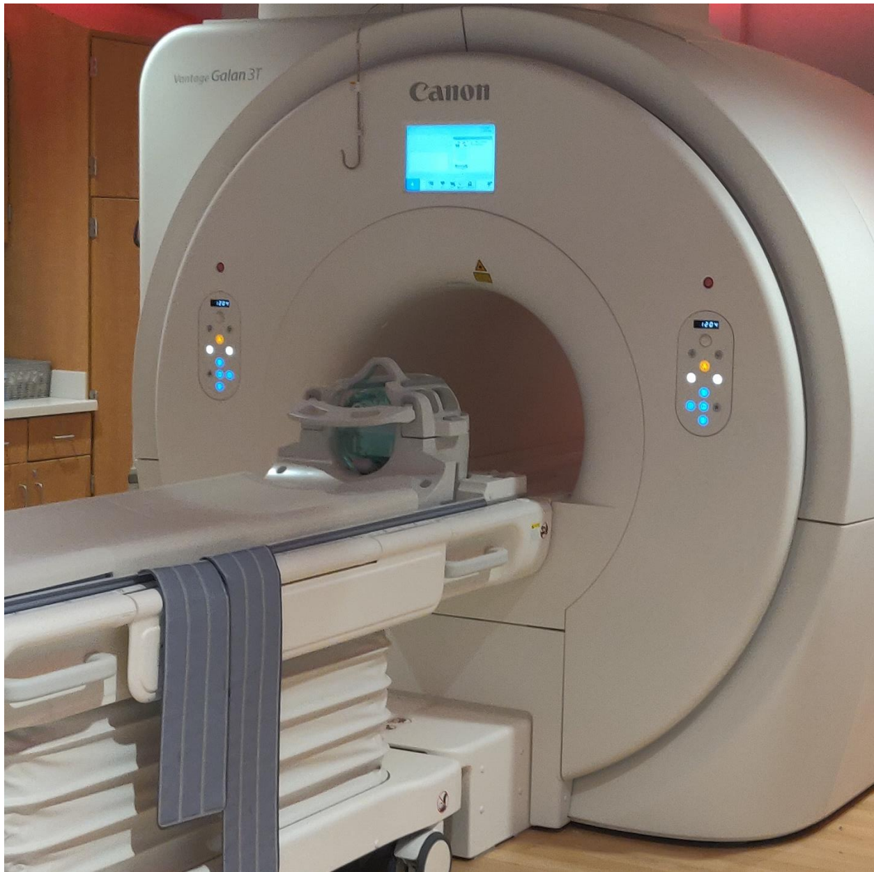
Figure 12. Photo of the large ACR MRI accreditation in the head receiver coil.
