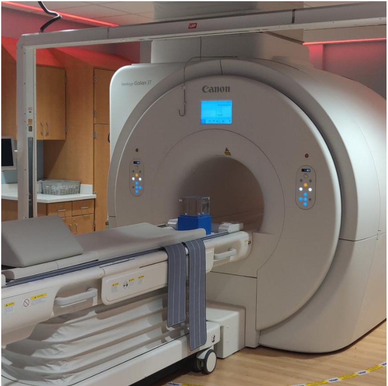
Figure 3: Photo of the daily QA phantom properly oriented on the MR-SIM patient couch.
