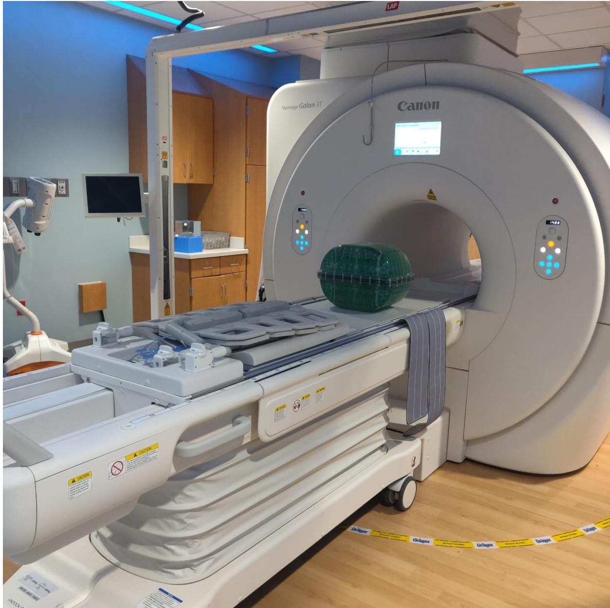
Figure 14. Photo of the assembled MagPhan RT on the patient couch.
