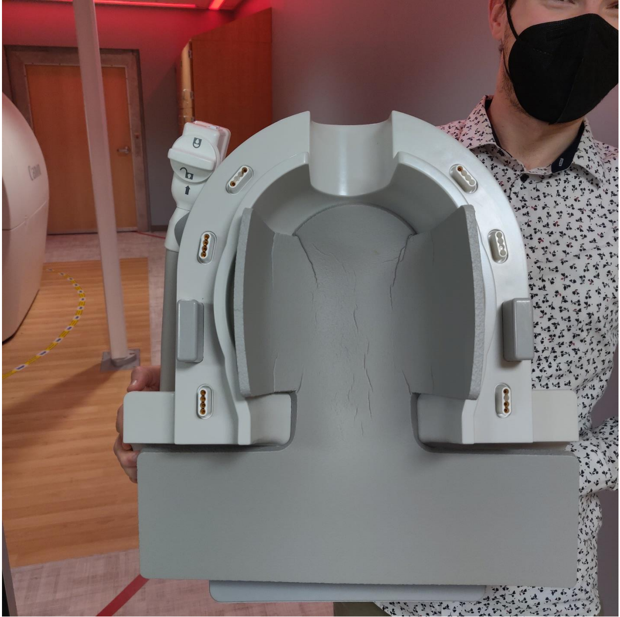
Figure 24. A photo of the base of the Atlas Head Neck coil and Atlas Cervical coil. The scanner “perceives” the coil as a different coil based on which top component is attached.
