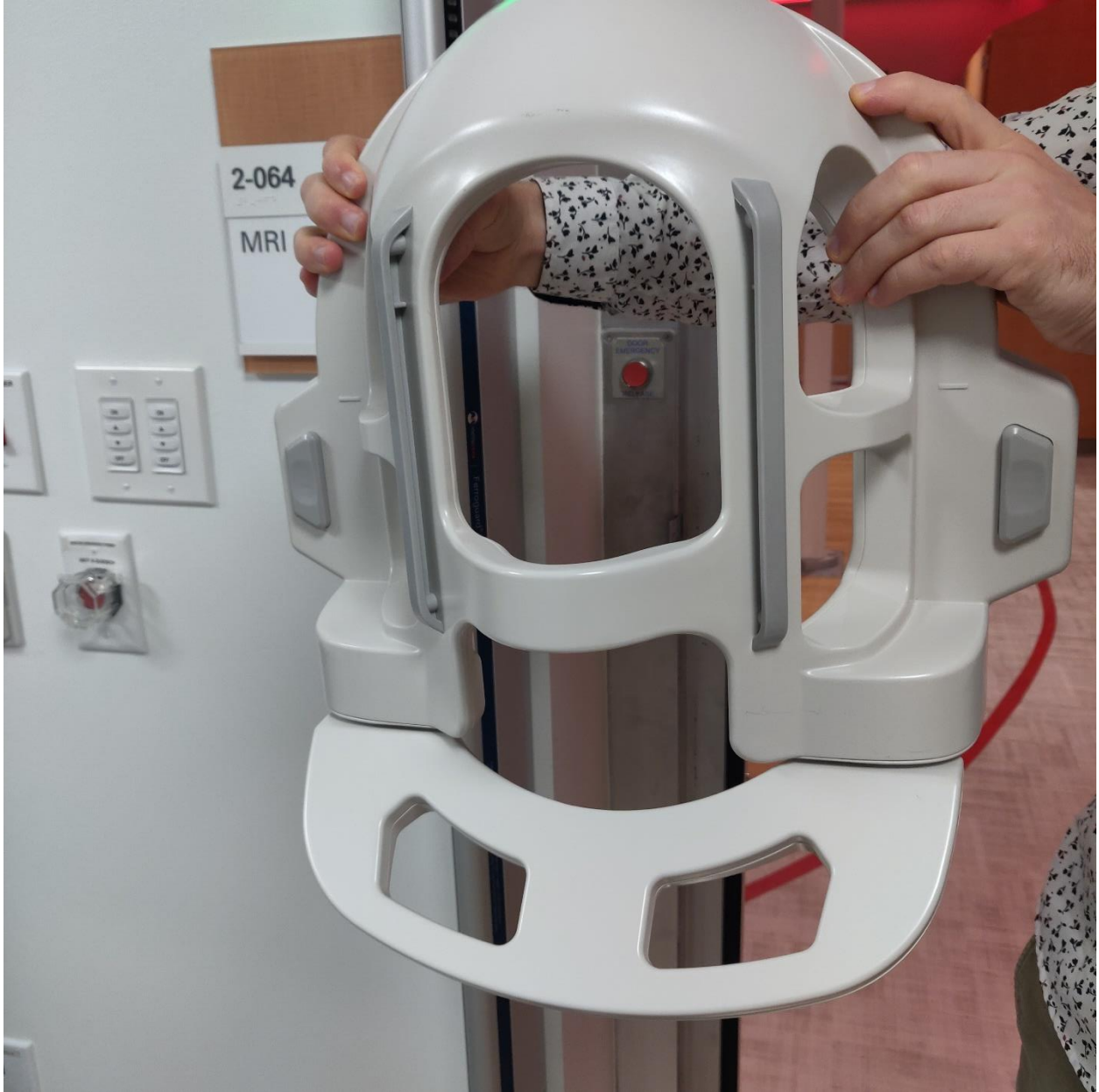
Figure 25. A photo of the top component of the Atlas Head Neck coil.
