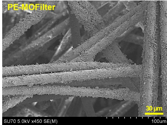
Figure 4. 4 SEM image of the deposition of p-BWO@MIL-1 particles on the fibers of MERV 13 electret media (PE-MOFilter).
