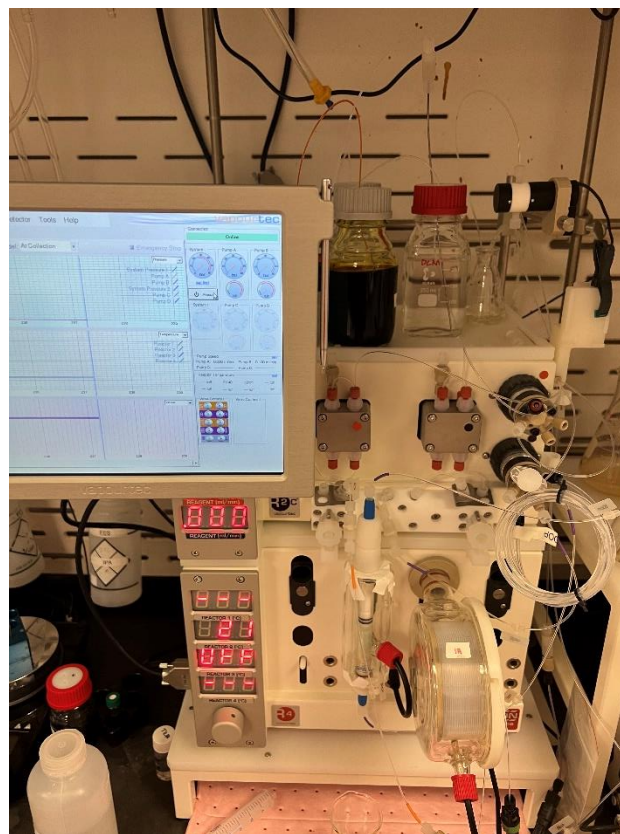
Figure 12. Image of an Example Plug Flow Reaction Instrument used in the Gupton Lab
