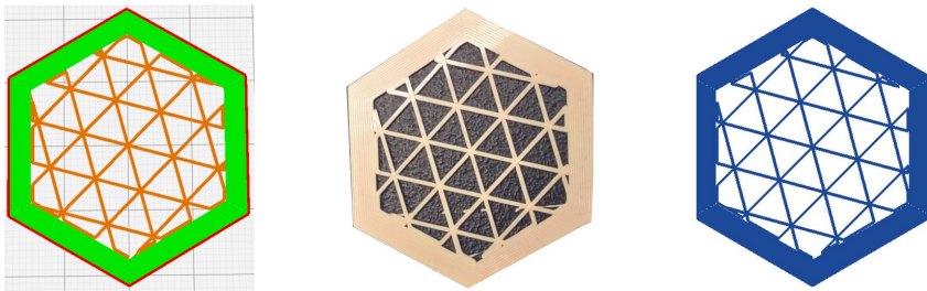
Fig. 71: Slicer representation (left), actual printed object (center), and accurate image recovered from FRoMEPP dataset (right)
