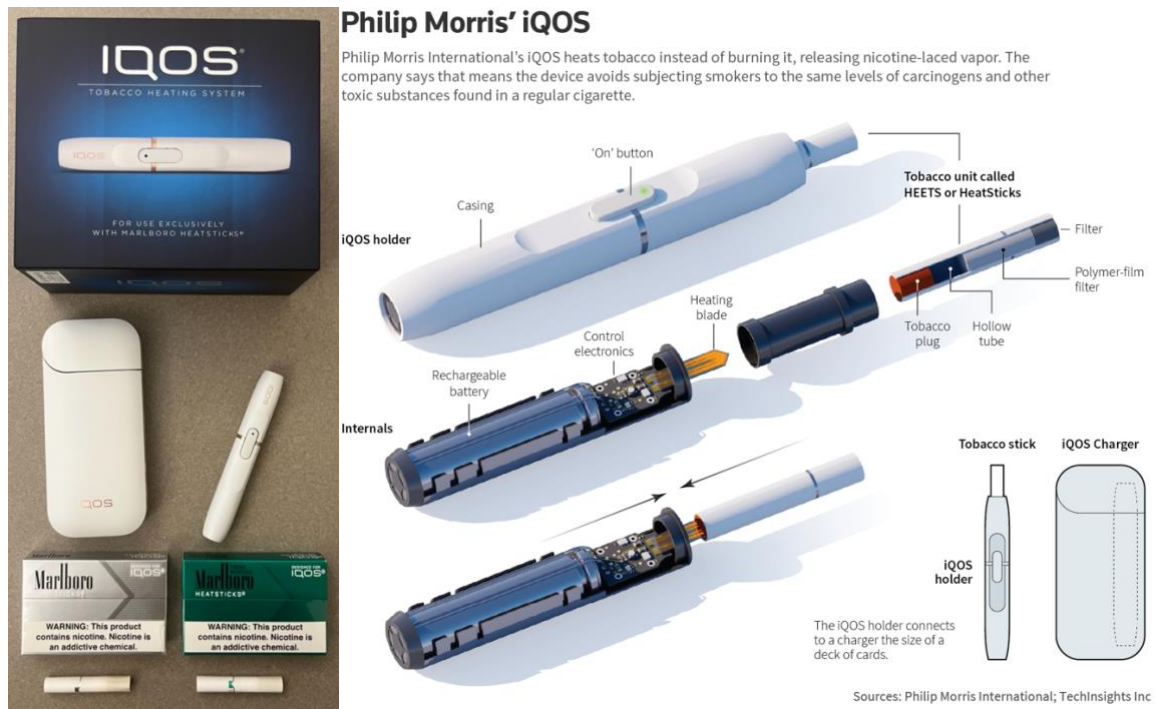
Figure 1. IQOS 2.4 tobacco heating system (left) and device schematic (right)
