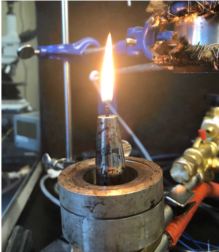
Figure 3.13: Oil vaporized and burned as it comes out of the center stainless steel tube. Note: preheated and ignited by flame from torch.
