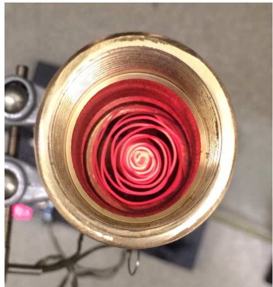
Figure 3.4: Combustion chamber with glowing ignition coil
