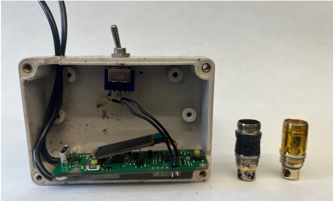
Figure 3.6: Evolv DNA 250 controller and 2 cotton coils. Note: they are wrapped in heat shrink, (Left) and in high temperature tape (right) and then had smaller holes added as an attempt to reduce the flow rate.
