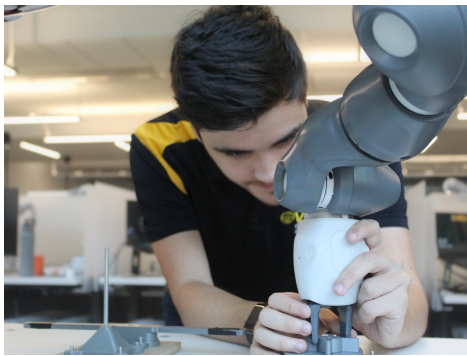
(a) Lead-through programming
