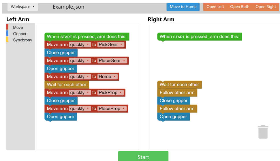
Figure 4.1: Interface of the Duplo programming language. Users can drag blocks from a toolbox on the left onto the programming canvases and attach them to existing blocks to create a program. Blocks that affect both arms are duplicated across canvases and vertically aligned.
