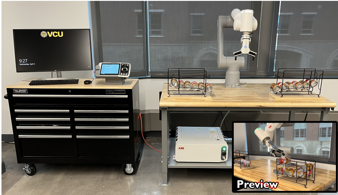
Figure 6.2: Experiment workspace. On the left, the desktop computer and the teaching pendant device are placed on a tool cart. On the right, the robot is fixed on a table along with the two dispensers randomly filled with cans containing two distinct flavors. At the bottom of the table, it is also possible to see the robot controller connected to the teaching pendant by a cable and a preview of the robot placing the can on the dispenser.
