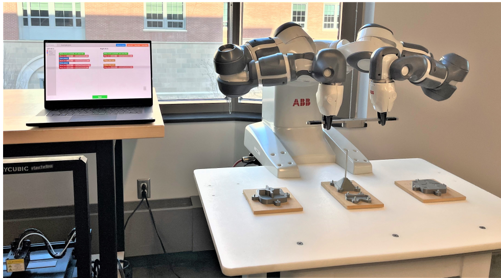
Figure 4.4: Experimental setup: Participants used a touch-screen-enabled laptop (left) to program a two-armed collaborative robot (right).
