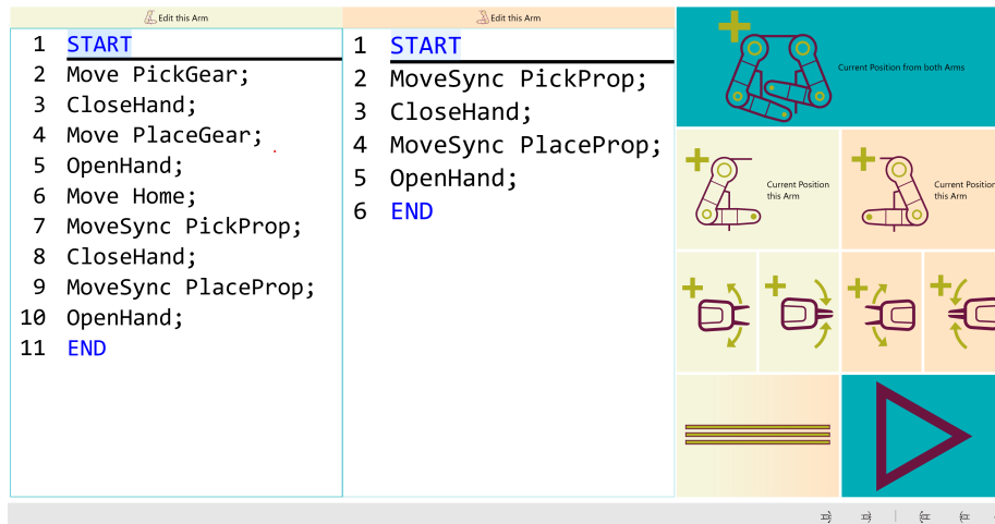
Figure 4.2: RobotStudio Online YuMi programming interface for two-armed robots: Two canvases show RAPID code for each arm side-by-side, with buttons allowing the quick insertion of commands into the code.
